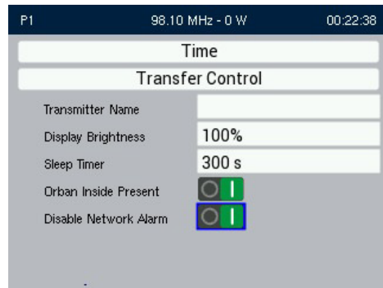
Disable Network Alarm enabled (network alarm suppressed)
