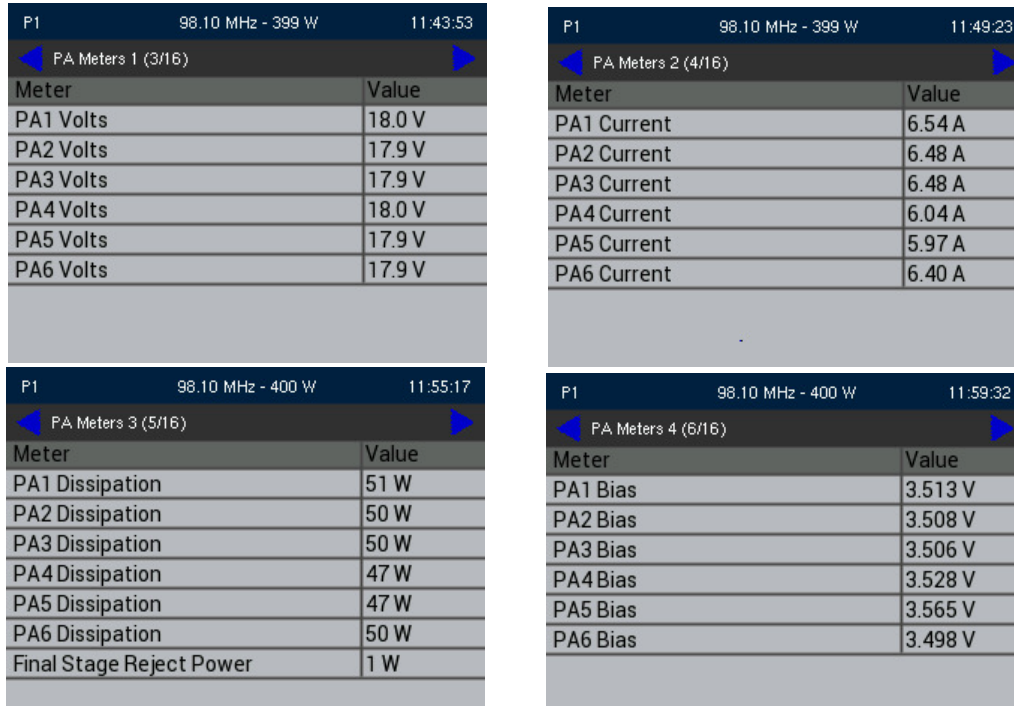
Figure 2.2.70: PA Meters (four screens shown for reference)
