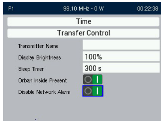
Disable Network Alarm enabled (network alarm suppressed)
