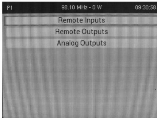
**Remote Inputs.** When you select Remote Inputs from the Remote I/O screen, you can edit parameters related to a Remote Input. See [Figure 2.2.116](#)).
