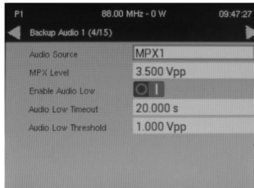
**NOTE:** *If you edit and save the Backup Audio settings after the transmitter switches over to the backup audio source due to a main audio source failure, the transmitter will switch back to the main audio source. If the main audio source is still in a failure state, the transmitter will switch back to the backup audio source, after the selected timeout period.*
