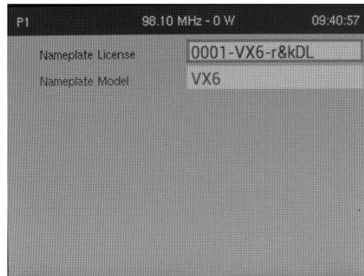
Use the Front Panel rotary knob to select the Nameplate License field and press the knob to enter the editing menu (see [Figure 2.2.135 on page 2.2.149](#)). Press the Back button to abort editing and return to the previous setting.
