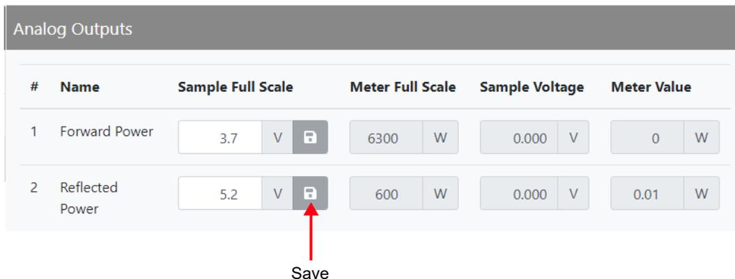
The values associated with each of these fixed meters are of a linear nature so that changes made to the Sample Full Scale field (allowable range is 1- 10 V, defaulted to 5 V) will be reflected in the other fields according to the following equation:
