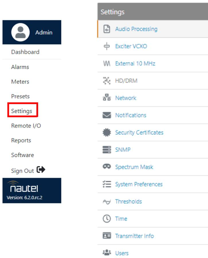
**NOTE:** For consistency the Settings menu is the same for all transmitter series. If a transmitter does not have a feature, such as Audio Processing or HD/DRM, that menu option is greyed out in the Settings list.
