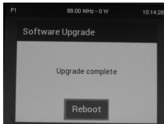
If an error is encountered during the upgrade procedure, a pop-up screen will be displayed indicating that the upgrade was unsuccessful and the Operating System will remain unchanged. Press Confirm to accept the failed upgrade and return the transmitter to the original (prior upgrade) operating system. See [Figure 2.4.4](#) on [page 2.4.5](#).
