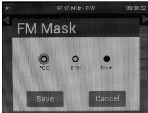
Use the Front Panel rotary knob to change the FM Mask setting. Press the Front Panel rotary knob to save the change. Press Cancel button to discard any changes and return to the previous menu.
