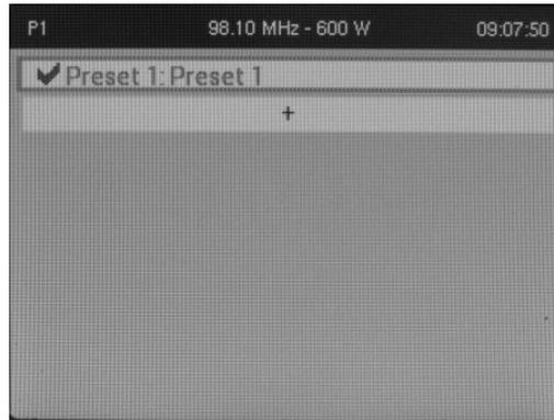
Use the Front Panel rotary knob to scroll through the existing presets. Press the Front Panel rotary knob to enable the preset as the transmitter’s active preset. Select Confirm to enable or Cancel to return to the previous menu.
