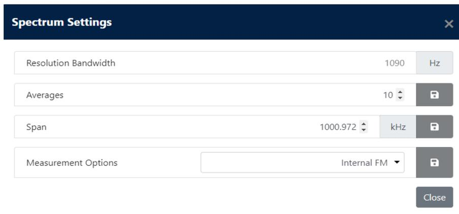
**NOTE:** The FM spectrum analyzer displays the ideal spectrum generated by the DSP. It is not necessarily the same as the spectrum seen at the RF output.
