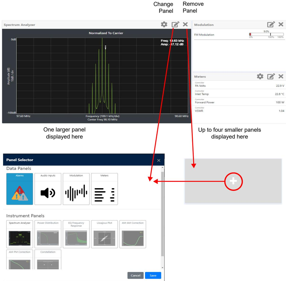
**NOTE:** For consistency the panel selector dialog is the same for all Nautel FM transmitters. If an instrument is greyed out, it is not currently available on the transmitter you are logged into.
