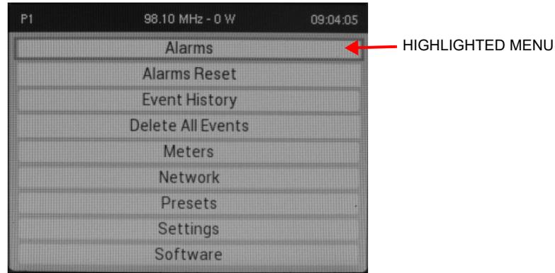
[Table 2.2.6](#) defines the available front panel display screens. Rotate the Front Panel rotary knob to select the desired function and press the knob to enable editing.
