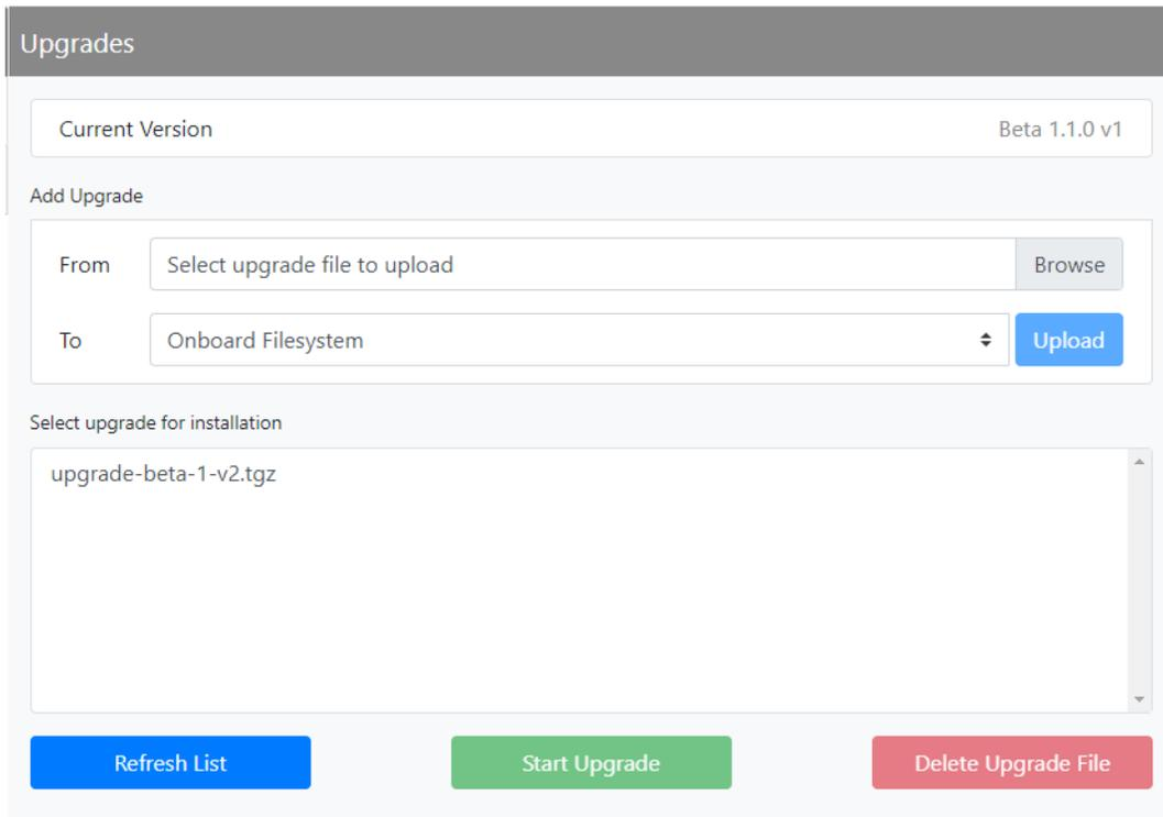
Select the upgrade file from the list and click Start Upgrade to initiate the software upgrade process. A warning will be displayed, indicating that the upgrade can take up to fifteen (15) minutes to complete and cannot be stopped once started. Also, the transmitter can remain in an on-air state during the upgrade. Press Yes to start the upgrade process or Cancel to not proceed with an upgrade. See [Figure 2.4.8](#).
