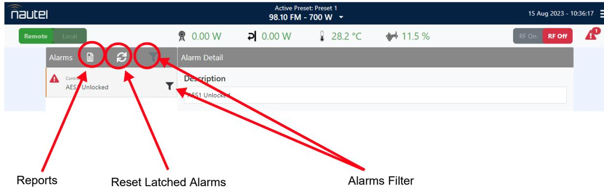
The Alarms page displays all active transmitter alarms. Alarms are listed by their host device (Controller or Exciter) and alarm name. Refer to the VX3 to VX6 Troubleshooting Manual for detailed information on alarm details such as root cause and troubleshooting tips.
