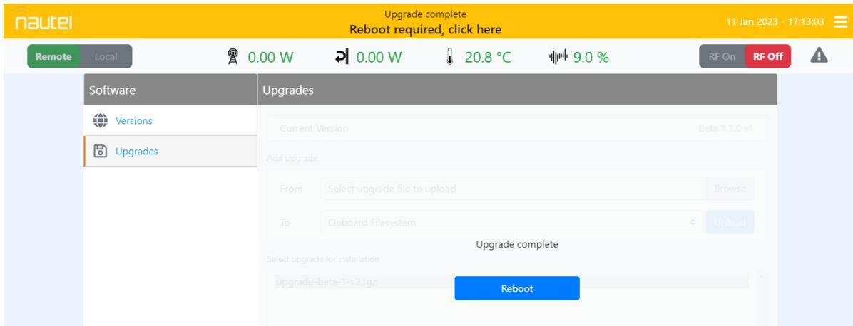
A warning will be displayed, indicating that the transmitter will be off-air for up to two (2) minutes during a reboot. Press Yes to reboot that transmitter or Cancel to revert to the previous software. See [Figure 2.4.11](#) on [page 2.4.9](#).
