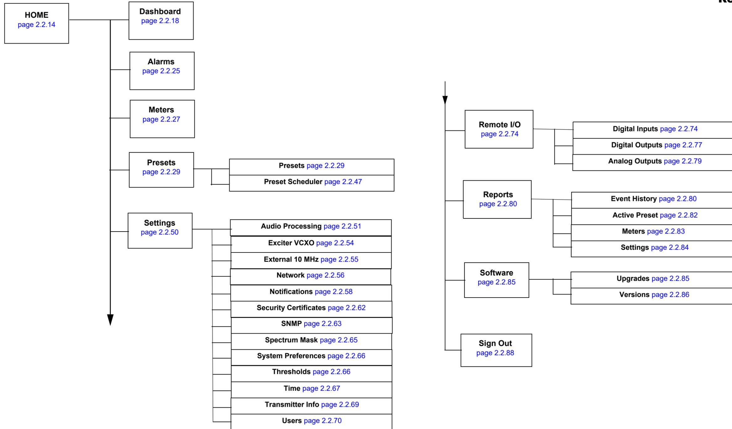
Figure 2.2.2: VX Transmitter AUI Flow Diagram
