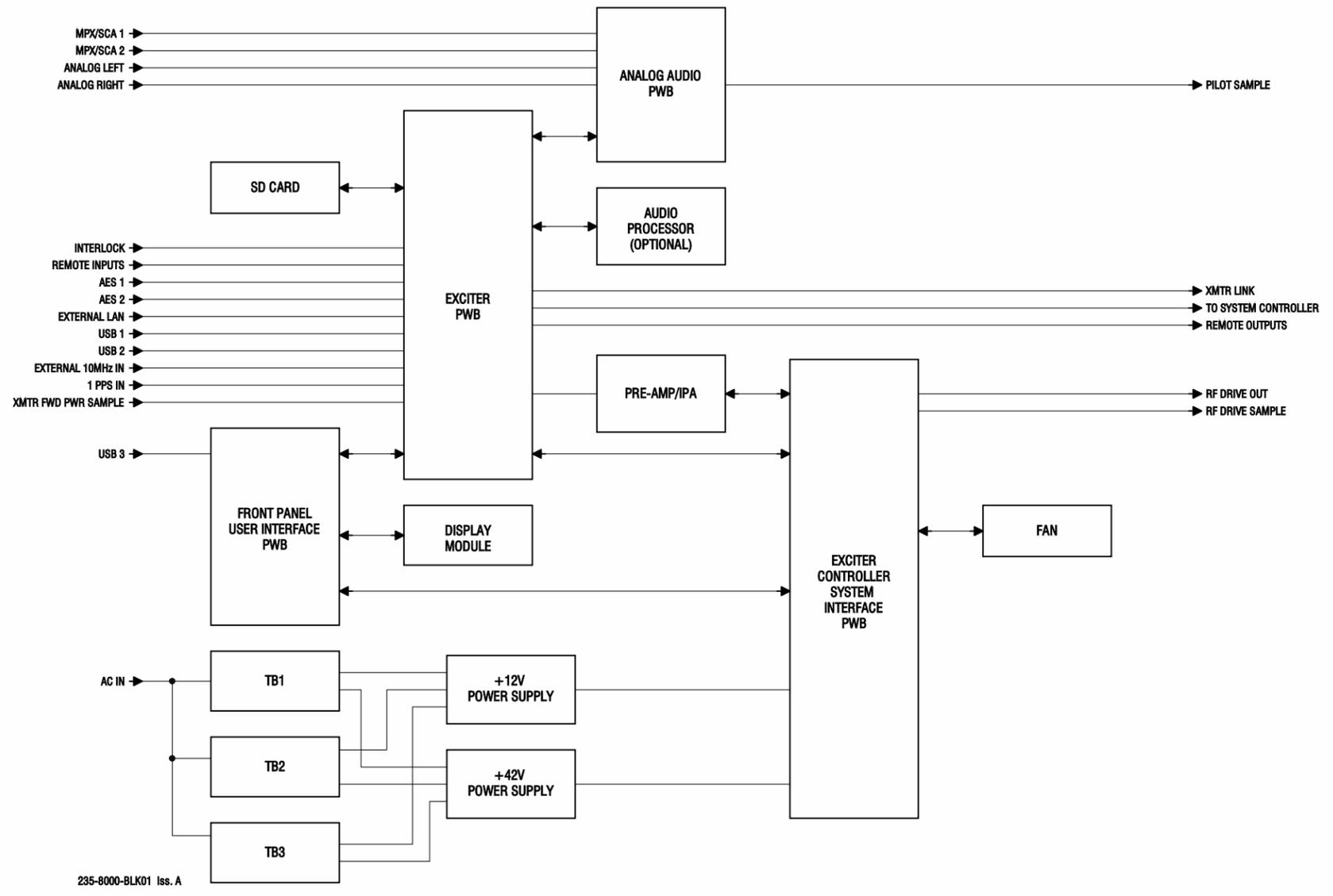
Figure 2.1.2: Block Diagram - Exciter/Controller Assembly
