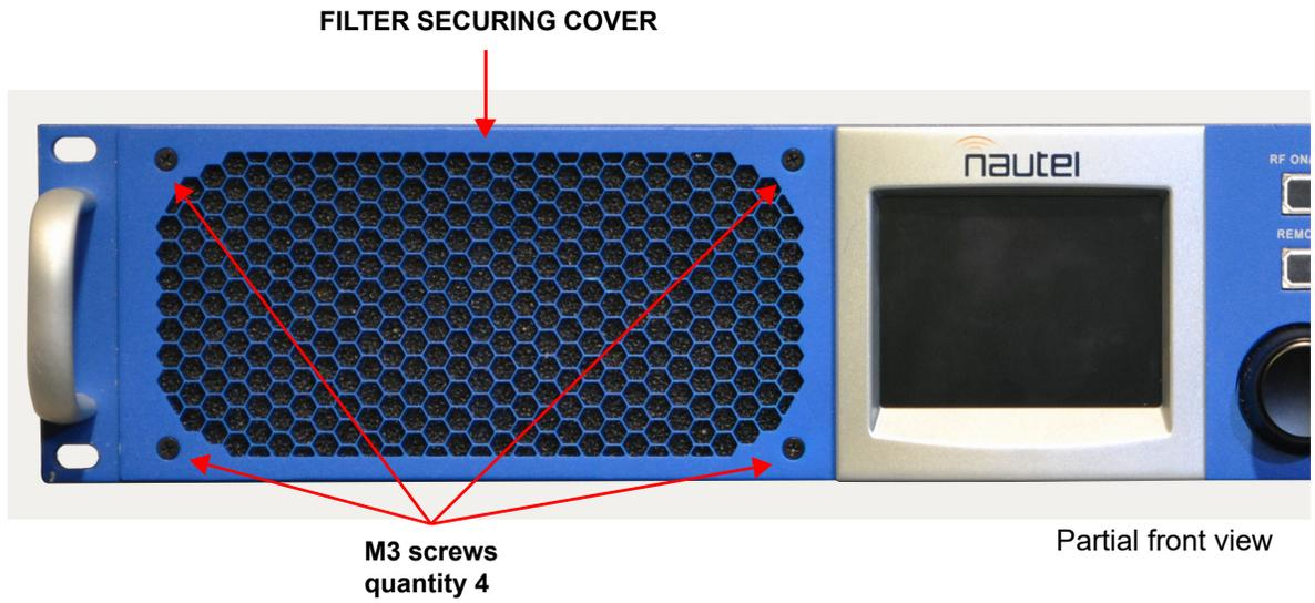
Figure 2.3.2: Replacing Amplifier Air Filter
