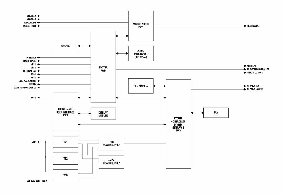
Figure 2.1.2: Block Diagram - Exciter/Controller Assembly
