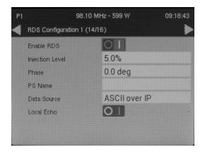
• UECP over IP (see Figure 2.2.92). Set the Injection Level.
