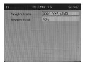
Use the Front Panel rotary knob to select the Nameplate License field and press the knob to enter the editing menu (see Figure 2.2.135 on page 2.2.149). Press the Back button to abort editing and return to the previous setting.
