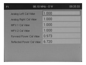
Use the Front Panel rotary knob to select the desired setting and press the knob to make changes. With the appropriate calibrated source applied, use the Front Panel rotary knob to set the new calibration value for the selected input. Press the Back button to discard any changes.
