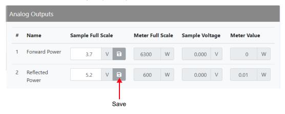
The values associated with each of these fixed meters are of a linear nature so that changes made to the Sample Full Scale field (allowable range is 1- 10 V, defaulted to 5 V) will be reflected in the other fields according to the following equation:
