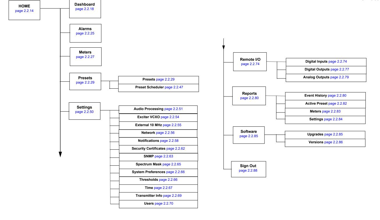
Figure 2.2.2: VX Transmitter AUI Flow Diagram
