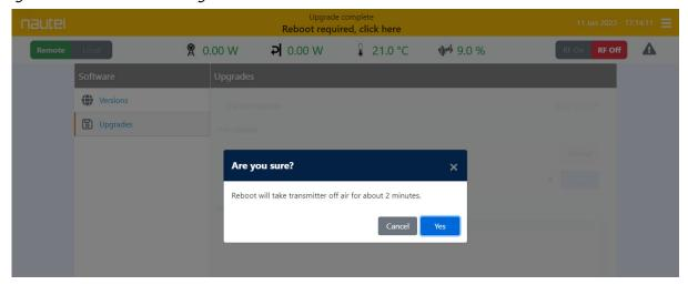
If the upgrade failed, the Operating System will remain unchanged and a pop-up screen will be displayed for the user to acknowledge the failed attempt.
