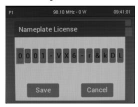
To enter a Nameplate License, use the Front Panel rotary knob to select the characters for the nameplate license name provided. Press the Front Panel rotary knob to save the changes. Press the Cancel button to discard the changes and return to the previous setting.
