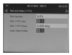
**NOTE**: *Pilot is not enabled with SCA or RDS. Pilot is only generated when the audio mode is stereo.*
