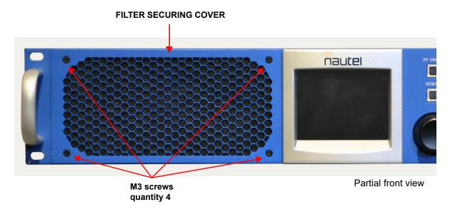
Figure 2.3.2: Replacing Amplifier Air Filter
