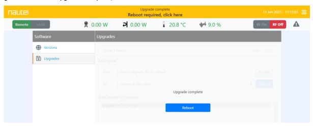
A warning will be displayed, indicating that the transmitter will be off-air for up to two (2) minutes during a reboot. Press Yes to reboot that transmitter or Cancel to revert to the previous software. See Figure 2.4.11 on page 2.4.9.
