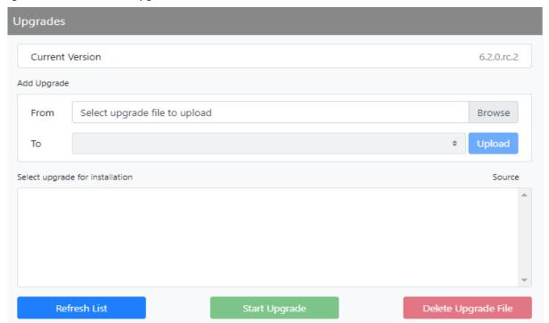
Select Browse to locate a .tgz file to upload to the transmitter and click Upload to save the file in the Select upgrade for installation field. A status bar will be displayed showing the percentage completed. See Figure 2.4.6.
