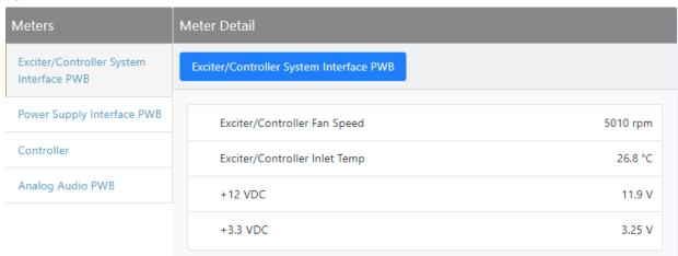
Exciter/Controller System Interface PWB Meter Detail shown for reference
