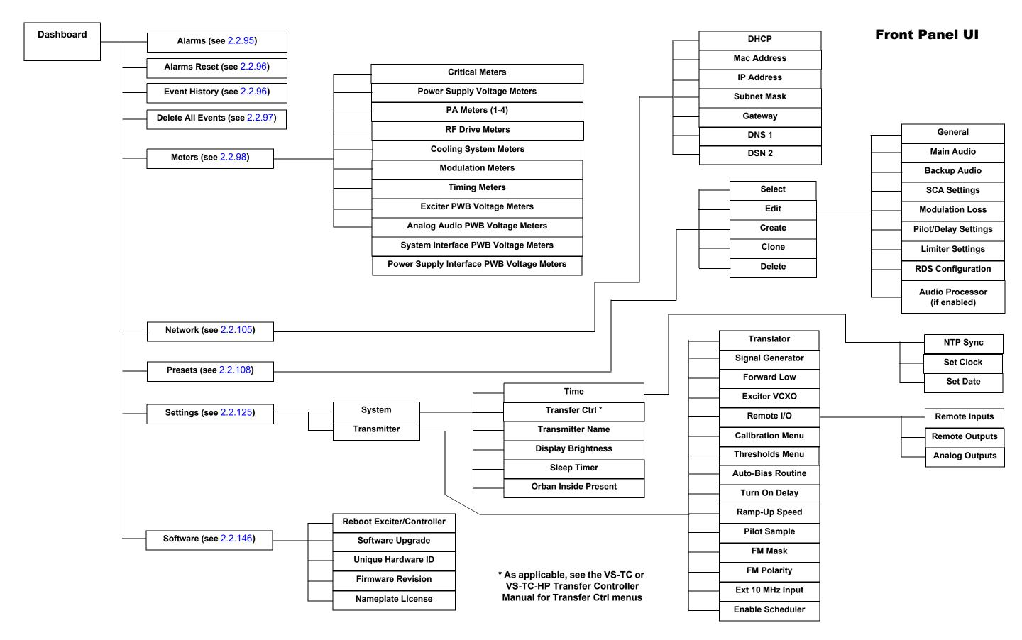
Figure 2.2.3: VX3 to VX6 Transmitter - Front Panel UI Menu Tree
