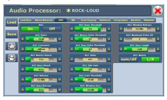
**NOTE**: The AGC Ratio range displays as Inf:1 to 2:1. Although you cannot set the AGC Ratio to Inf:1 (it will default to 4:1), some Orban presets are defaulted for an Inf:1 setting. Nautel recommends you edit the setting to an appropriate ratio (4:1, 3:1 or 2:1).
