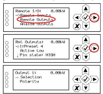
Use the up and down buttons to select the desired remote output (1 through 16) from the list. Each screen shows the current digital output parameter (e.g., RF On/Off), as well as the polarity (e.g., RF On = Low) and current state (e.g., high, low) of the corresponding output pin. Use the right-arrow button to enter the **Selection/Polarity** screen for the selected output to allow editing of the selection or the polarity. Press cancel (X) to return to the previous menu.
