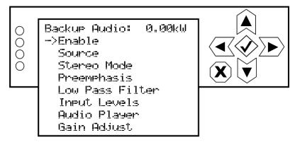
Use the up and down buttons to scroll through the backup audio menu options, then press the accept (checkmark) or right arrow button to enter the selected editing screen. With the exception of the **Enable** screen (select ON to enable, OFF to disable), the editing screens for the **Backup Audio** menu are the same as the **Main Audio** menu (see Figure 2.57 on page 2-80). Press the cancel (X) button to discard changes and return to the previous menu.
