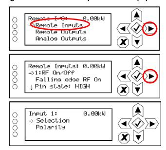
Use the up and down buttons to select the desired remote input (1 through 10) from the list. Each screen shows the current remote input parameter (e.g., RF On/Off), as well as the polarity (e.g., Falling edge RF On) and current state (e.g., high, low) of the corresponding input pin. Use the right-arrow button to enter the Selection/Polarity screen for the selected input to allow editing of the selection or the polarity. Press cancel (X) to return to the previous menu.
