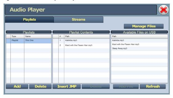
The playlist (or Shoutcast/Livewire stream) is typically used as an audio loss backup. For example, the user may operate with Preset 1 using one of the standard audio sources. Preset 1 can be configured to switch to another preset (e.g., Preset 2), which uses a playlist or stream, if Preset 1 loses its audio. See "Changing the OS Password" on page 4-4 for more information.
