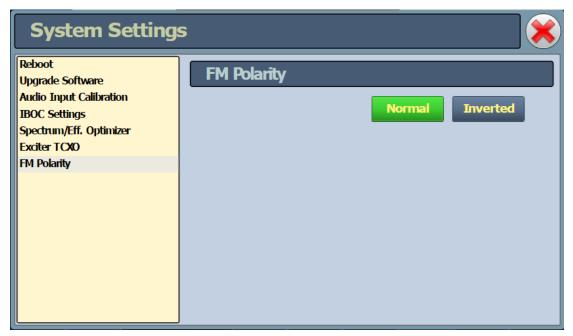
Select either **Normal** (default; positive going modulation signal yields negative deviation) or **Inverted** (positive going modulation signal yields positive deviation) and confirm your setting when prompted.
