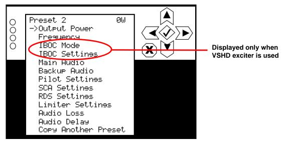
Within the preset editing menu, use the up and down buttons to scroll through the options and press the accept (checkmark) button to enter the selected editing menu/screen. Press the cancel (X) button to return to the previous menu. Parameters that can be edited are:
