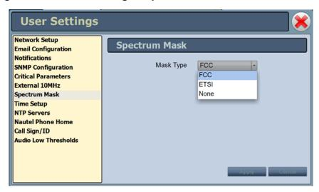
Use the Mask Type pull down menu to select the appropriate mask standard (the factory setting is FCC). Press the Apply button to save the change or press Cancel to discard changes.
