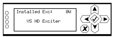
Use the up and down buttons to select the appropriate exciter configuration - Internal VS Exciter, VS HD Exciter or External FM Exciter. Press the accept (checkmark) button to save the change. Press X to abort the change and return to the previous menu.
