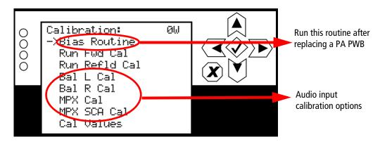
**RUNNING THE BIAS ROUTINE.** You must run the transmitter's bias routine immediately after installation of a new PA PWB.
