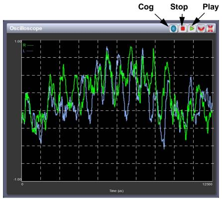
Figure 2.29: Oscilloscope (Left/Right Audio input shown)
