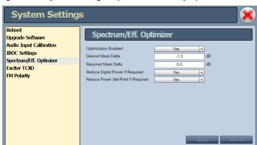
Figure 2.87: System Settings - Spectrum/Efficiency Optimizer
