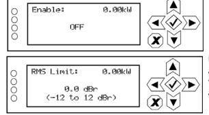
Use the up and down arrows to select ON or OFF, then press the accept (checkmark) button to save the change. Press the cancel (X) button to discard changes and return to the previous menu. Default selection is OFF.
