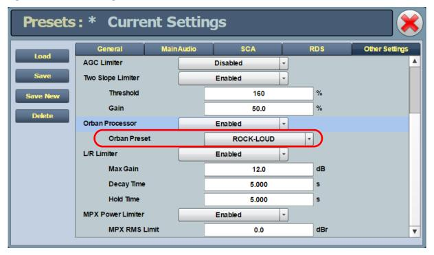
Figure 2.161: Enabling the Orban Audio Processor - Remote AUI
