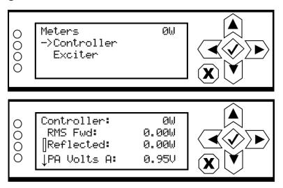
Use the up and down buttons to select Controller or Exciter and then scroll through the appropriate list of metered parameters shown below:
