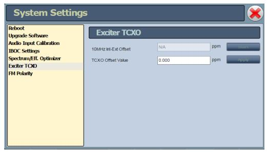
To automatically calibrate the internal reference for the exciter, click the **Start** button. The progress bar at the bottom of the page will indicate that the calibration is in progress or complete. The **TCXO Offset Value** will appear when calibration is complete. Alternatively, if the required offset value is known, you can manually enter it in the **TCXO Calibration Value** field and click the **Apply** button.
