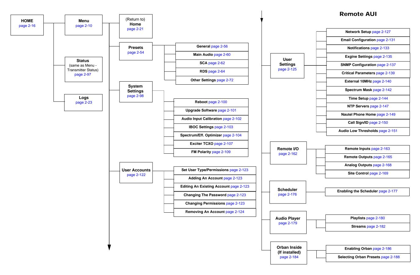
Figure 2-3: VS Transmitter AUI Flow Diagram
