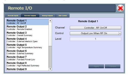
Select the desired remote output (1 through 16) from the list. The **Channel** and **Logic** settings for the selected output, as well as the current logic level (1 or 0), are displayed on the right-hand side of the page. You can define the **Channel** and **Logic** settings as follows:
