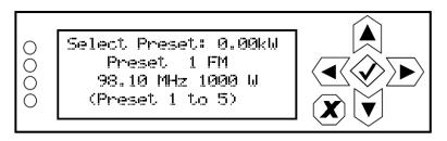
Use the up and down buttons to scroll through the existing presets. Press the accept (checkmark) button to enable the preset as the transmitter's active preset. Press the cancel (X) button to return to the previous menu.
