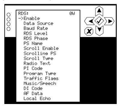
Use the up and down buttons to move the cursor to the desired RDS setting and then press the right button to enable editing of the parameter.
