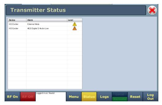
The Transmitter Status page displays all active transmitter alarms. Alarms are listed by their host device (Controller or Exciter), alarm name and severity level [a single orange! indicates low severity (RF output not affected); a single red! indicates medium severity (RF output is reduced); three red! indicates high severity (RF output is inhibited)]. Refer to the VS2.5 Troubleshooting Manual for detailed information on alarm details such as root cause and troubleshooting tips.
