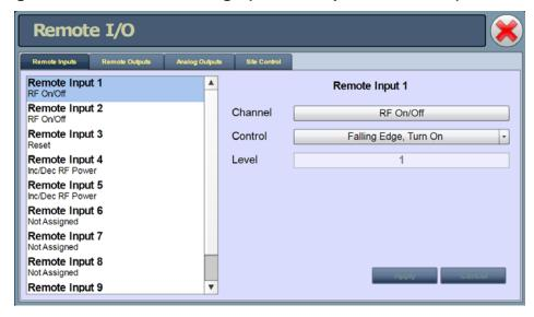
Select the **Remote Inputs** (see Remote Inputs - AUI on page 2-163) or **Remote Outputs** (see Remote outputs - AUI on page 2-165) tab to view or edit detail on the remote inputs or outputs.
