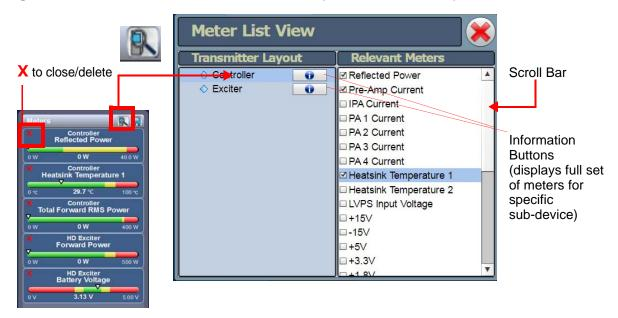
Figure 2.36: VSHD Meter List View Window (Controller Shown)
