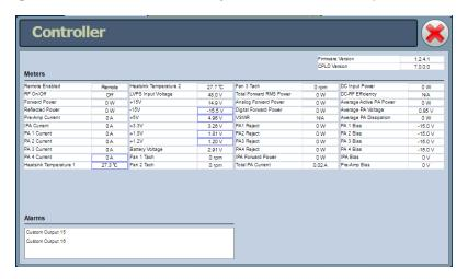
Figure 2.37 displays the status of the selected sub-system, as well as real-time meter values. The Alarms section shows any active alarms pertaining to the sub-system.
