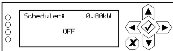
Use the up and down buttons to select **ON** (enable) or **OFF** (disable). The default setting is **OFF**. Press cancel (**X**) to return to the previous menu.
