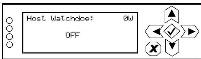
Use the up and down buttons to toggle between **OFF** and **ON**. Press the accept (checkmark) button to save the change. Press cancel (**X**) to discard changes and return to the previous menu.
