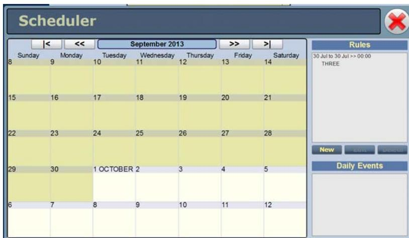
The left-hand side of the **Scheduler** page displays a monthly calendar (e.g., September 2013). Use the << and >> buttons to navigate between months. Use the < and > buttons to navigate to the beginning and the end of the schedule.
