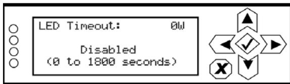
Select disabled (i.e., no timeout) or select a time period between 0 and 1800 seconds (30 minutes) (in 5 s increments). Press the cancel (X) button to discard changes and return to the previous menu. Default setting is 900 s (15 minutes).
