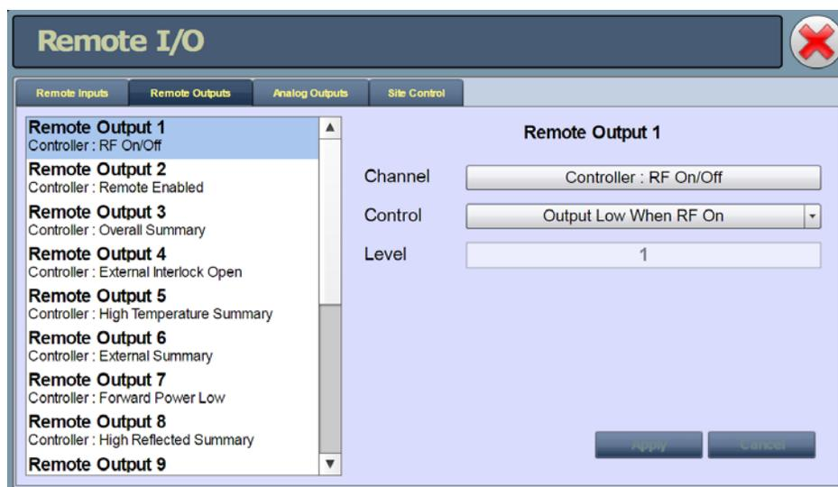
Select the desired remote output (1 through 16) from the list. The **Channel** and **Logic** settings for the selected output, as well as the current logic level (1 or 0), are displayed on the right-hand side of the page. You can define the **Channel** and **Logic** settings as follows:
