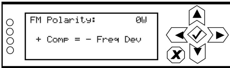
Use the up and down buttons to toggle between **+ Comp = - Freq Dev** and **+ Comp = + Freq Dev**. The default setting is **+ Comp = - Freq Dev**. Press the accept (checkmark) button to save the change. Press **X** to abort the change and return to the previous menu.
