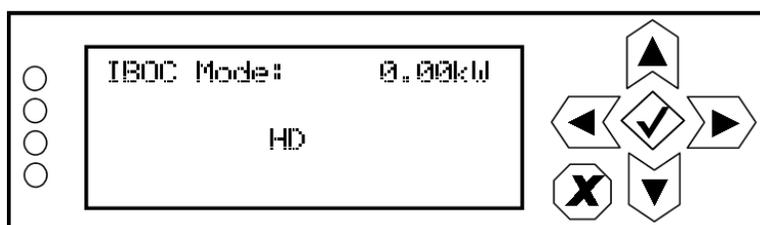
**IBOC SETTINGS.** When you select IBOC Settings from the **Preset** editing options screen (viewable only when IBOC Mode is set to HD or FM+HD), you can edit various IBOC parameters (see [Figure 2.54](#)).
