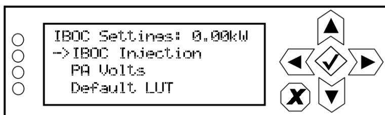
Use the up and down buttons to scroll through the main audio menu options, then press the accept (checkmark) or right arrow button to enter the selected editing screen. [Figure 2.55](#) shows the editing screens for the **IBOC Settings** menu. Press the cancel (X) button to discard changes and return to the previous menu.
