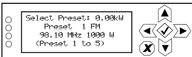
Use the up and down buttons to scroll through the existing presets. Press the accept (checkmark) button to enable the preset as the transmitter's active preset. Press the cancel (X) button to return to the previous menu.
