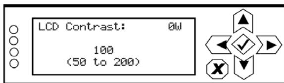
Select a value between 50 (lighter contrast) and 200 (darker contrast) (in increments of 5). Press the cancel (X) button to discard changes and return to the previous menu. Default setting is 100.
