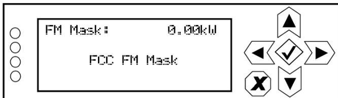
Use the up and down buttons to toggle between **FCC FM Mask**, **ETSI FM Mask** and **No FM Mask**. The factory setting is **FCC FM Mask**. Press the accept (checkmark) button to save the change. Press cancel (X) to discard changes and return to the previous menu.
