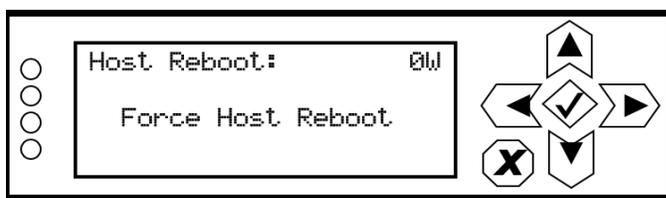
Use the up and down buttons to toggle between **Force Host Reboot** and **Cancel**. Press the accept (checkmark) button to save the change. If a reset is selected, it will occur immediately. Select **Cancel** or press **X** to abort the reset and return to the previous menu.
