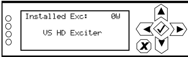
Use the up and down buttons to select the appropriate exciter configuration - Internal VS Exciter, VS HD Exciter or External FM Exciter. Press the accept (checkmark) button to save the change. Press X to abort the change and return to the previous menu.
