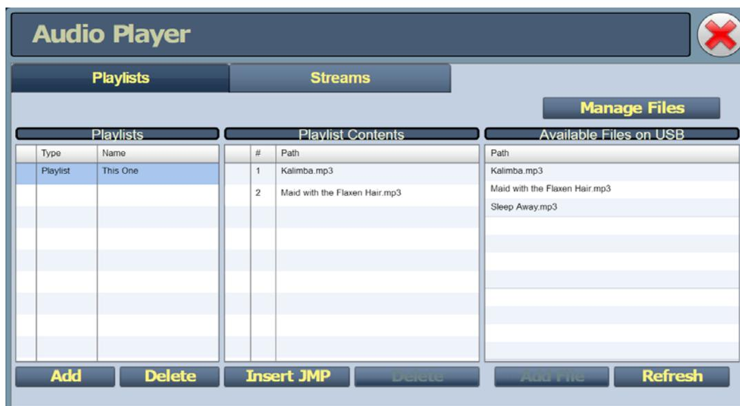
The playlist (or Shoutcast/Livewire stream) is typically used as an audio loss backup. For example, the user may operate with Preset 1 using one of the standard audio sources. Preset 1 can be configured to switch to another preset (e.g., Preset 2), which uses a playlist or stream, if Preset 1 loses its audio. See [“Changing the OS Password” on page 4-4](#) for more information.
