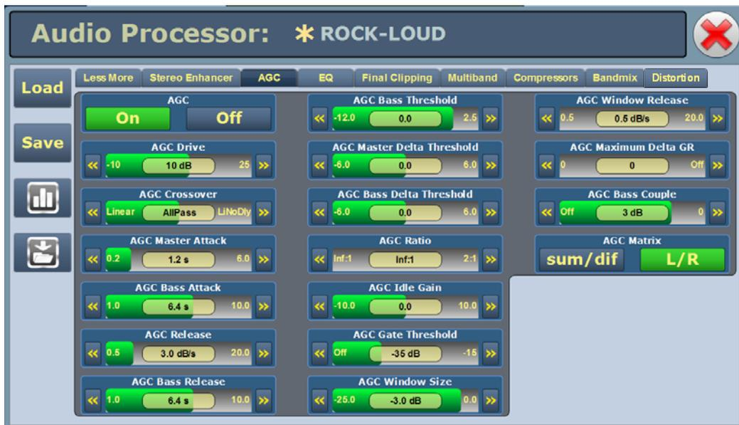
**NOTE:** The AGC Ratio range displays as Inf:1 to 2:1. Although you cannot set the AGC Ratio to Inf:1 (it will default to 4:1), some Orban presets are defaulted for an Inf:1 setting. Nautek recommends you edit the setting to an appropriate ratio (4:1, 3:1 or 2:1).
