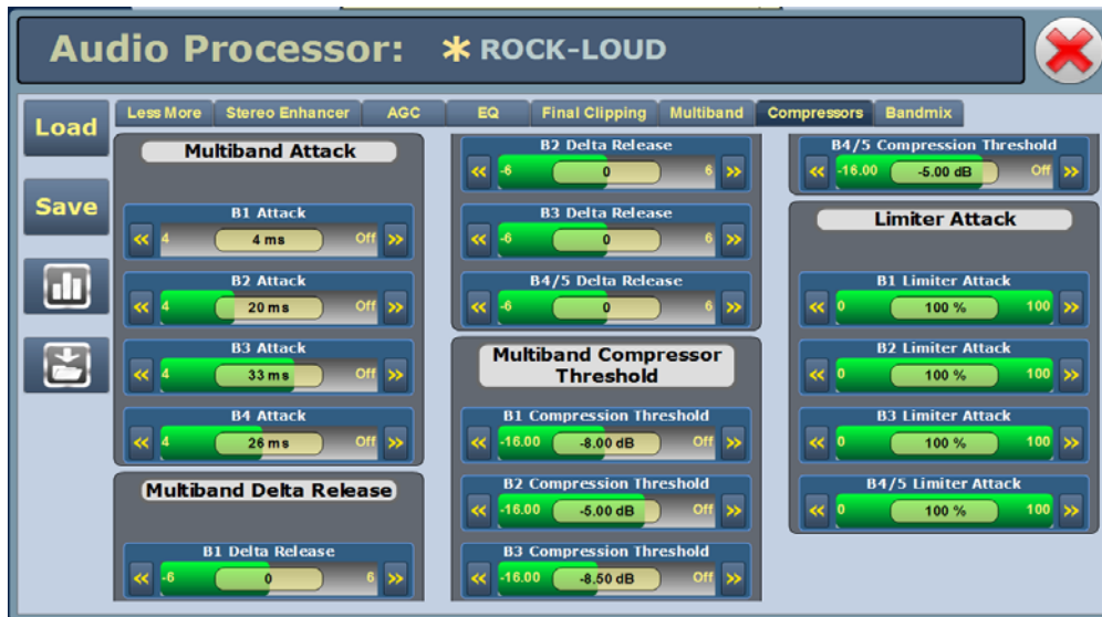
Figure 2.173: Audio Processor Menu - Compressors Tab
