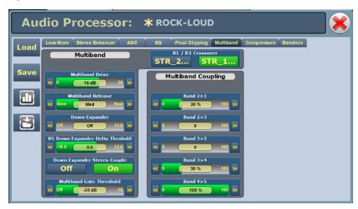
Figure 2.159: Audio Processor Menu - Multiband tab
