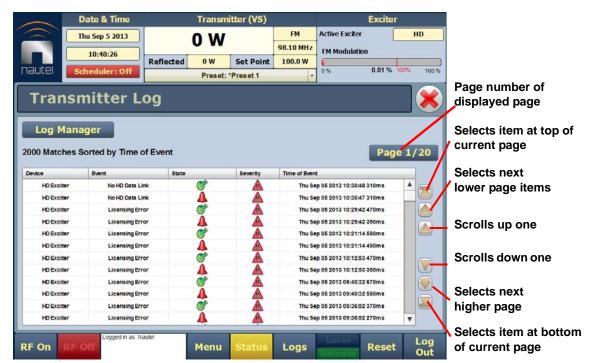
The main screen displays a chronological listing of events. Depending on the selections made in the **Log Manager** screen (see Managing the log on page 2-24), the events displayed may be filtered by the originating device (Controller or Exciter), and the time of occurrence.
