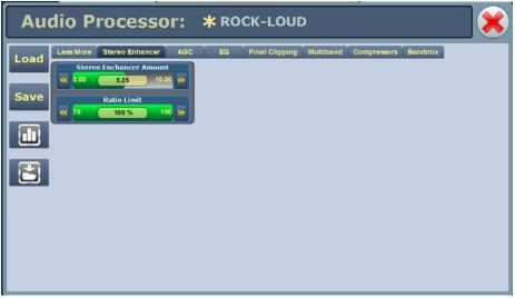
Figure 2.155: Audio Processor Menu - Stereo Enhancer tab
