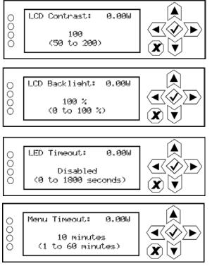
Select a value between 50 (lighter contrast) and 200 (darker contrast) (in increments of 5). Press the cancel (X) button to discard changes and return to the previous menu. Default setting is 100.
