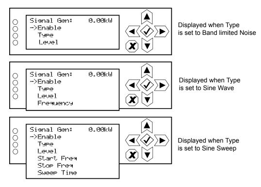
Use the up and down buttons to move the cursor to the desired line item and then press the right button to enable editing.
