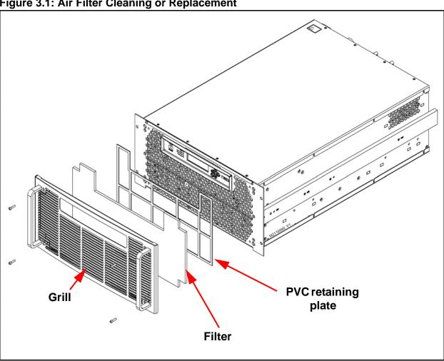
Figure 3.1: Air Filter Cleaning or Replacement
