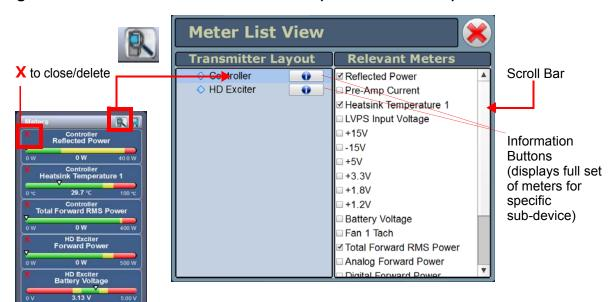
Figure 2.33: VSHD Meter List View Window (Controller Shown)
