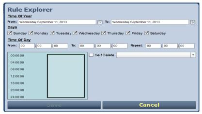
When you click in the Rules list, you have the option to edit or delete an existing rule, or to create a new rule. Click the **New** or **Edit** button to display the **Rule Explorer** window (see Figure 2.139 on page 2-155). Click **Delete** to remove a rule from the list.
