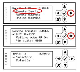
Use the up and down buttons to select the desired digital input (1 through 10) from the list. Each screen shows the current digital input parameter (e.g., **RF On/Off**), as well as the polarity (e.g., **Falling edge RF On**) and current state (e.g., high, low) of the corresponding input pin. Use the right-arrow button to enter the **Selection/Polarity** screen for the selected input to allow editing of the selection or the polarity. Press cancel (**X**) to return to the previous menu.
