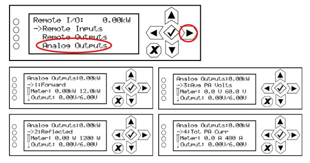
Use the up and down buttons to select the desired analog output (1 through 4) from the list. Each screen shows the analog output parameter (e.g., Forward Power, Reflected Power, Avg PA Volts or Total PA Current), as well as the meter reading (actual and full-scale) and the output pin voltage (actual and full-scale). Press cancel (X) to return to the previous menu.
