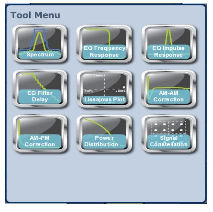
The AM-AM Correction, AM-PM Correction and Power Distribution tool menu icons appear only when the transmitter is operating with a VSHD exciter.
