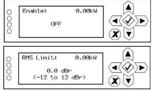
Use the up and down arrows to select ON or OFF, then press the accept (checkmark) button to save the change. Press the cancel (X) button to discard changes and return to the previous menu. Default selection is OFF.
