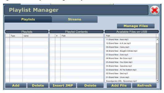
The playlist (or Shoutcast/Livewire stream) is typically used as an audio loss backup. For example, the user may operate with Preset 1 using one of the standard audio sources. Preset 1 can be configured to switch to another preset (e.g., Preset 2), which uses a playlist or stream, if Preset 1 loses its audio. See "Configuring a Mod Loss Backup Preset" on page 4-4 for more information.
