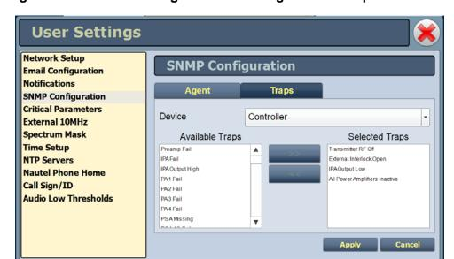
Figure 2.104: User Settings - SNMP Configuration - Traps Tab
