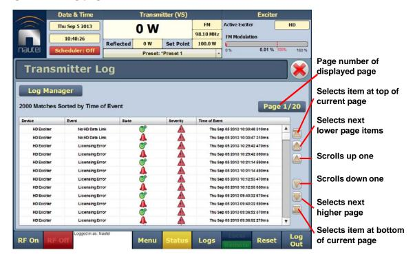
The main screen displays a chronological listing of events. Depending on the selections made in the **Log Manager** screen (see Managing the log on page 2-24), the events displayed may be filtered by the originating device (Controller or Exciter), and the time of occurrence.
