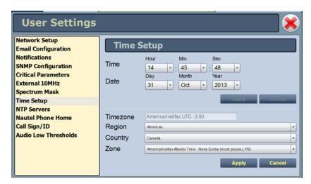
The **Time Setup** option allows users to set the exact time and date information as well as regional and timezone settings for a transmitter location.
