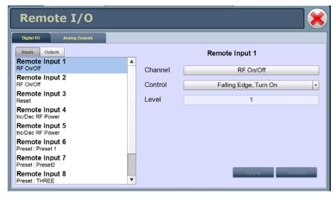
Click the **Inputs** (see Digital inputs - AUI on page 2-145) or **Outputs** (see Digital outputs - AUI on page 2-147) tab to view or edit detail on the digital inputs or outputs.
