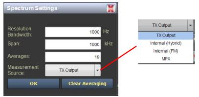
Note: The FM spectrum analyzer displays the ideal spectrum generated by the DSP. It is not necessarily the same as the spectrum seen at the RF output.
