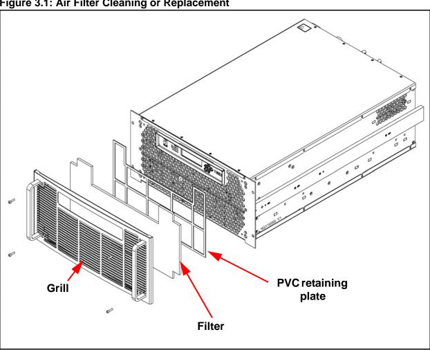
Figure 3.1: Air Filter Cleaning or Replacement
