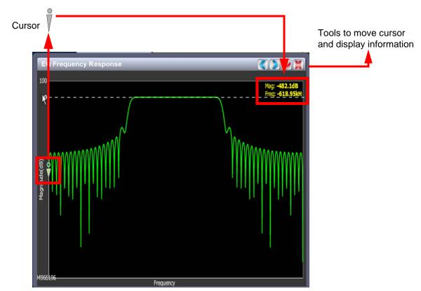
Figure 2.20: Instrument Cursor Manipulation
