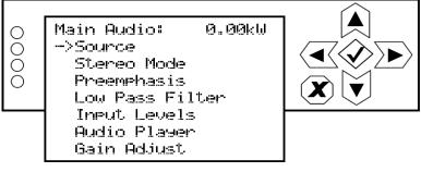
Use the up and down buttons to scroll through the main audio menu options, then press the accept (checkmark) or right arrow button to enter the selected editing screen. Figure 2.56 shows the editing screens for the Main Audio menu. Press the cancel (X) button to discard changes and return to the previous menu.
