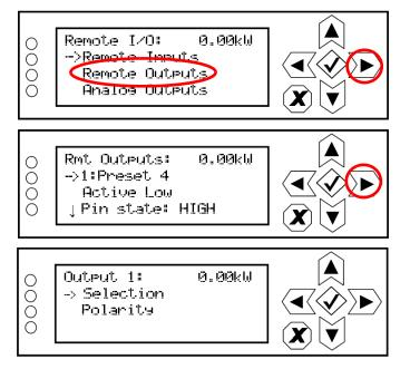
Use the up and down buttons to select the desired digital output (1 through 16) from the list. Each screen shows the current digital output parameter (e.g., RF On/Off), as well as the polarity (e.g., RF On = Low) and current state (e.g., high, low) of the corresponding output pin. Use the right-arrow button to enter the **Selection/Polarity** screen for the selected output to allow editing of the selection or the polarity. Press cancel (X) to return to the previous menu.
