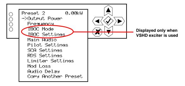
Within the preset editing menu, use the up and down buttons to scroll through the options and press the accept (checkmark) button to enter the selected editing menu/screen. Press the cancel (X) button to return to the previous menu. Parameters that can be edited are:
