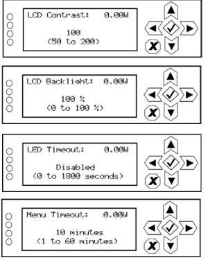
Select a value between 50 (lighter contrast) and 200 (darker contrast) (in increments of 5). Press the cancel (X) button to discard changes and return to the previous menu. Default setting is 100.
