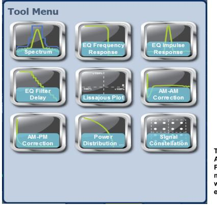
The AM-AM Correction, AM-PM Correction and Power Distribution tool menu icons appear only when the transmitter is operating with a VSHD exciter.
