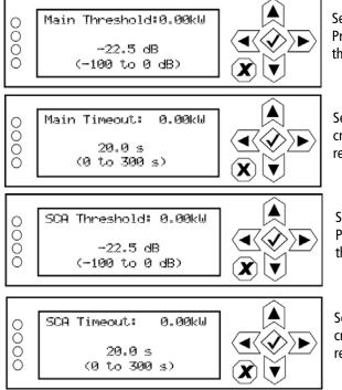
Select a level between -100 and 0 dB (in 0.5 dB increments). Press the cancel (X) button to discard changes and return to the previous menu. Default setting is -22.5 dB.
