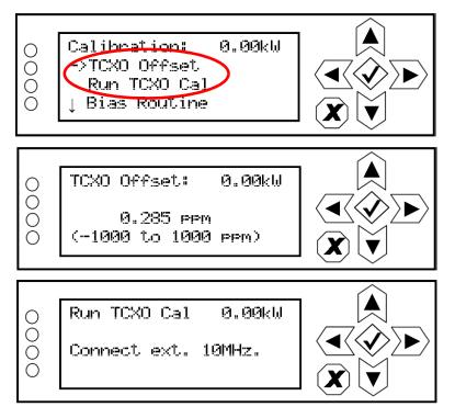
Use the up or down arrow to place the cursor next to **TCXO Offset**, then press the accept (checkmark) button to enter the **TCXO Offset** screen. Use the up and down arrows to set the TCXO offset value (in ppm) for the external 10 MHz source. When complete, press the accept (checkmark) button to save the change. Press cancel (**X**) to discard changes and return to the previous menu.
