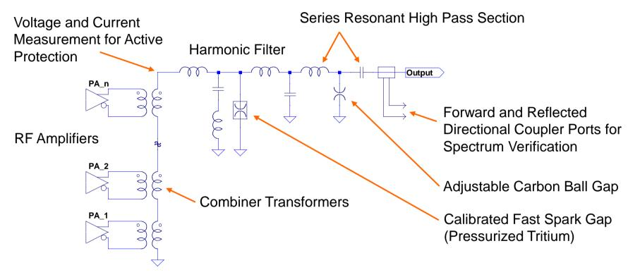
Frequency Agile: Harmonic Filter Re-Tune in a Few Hours
