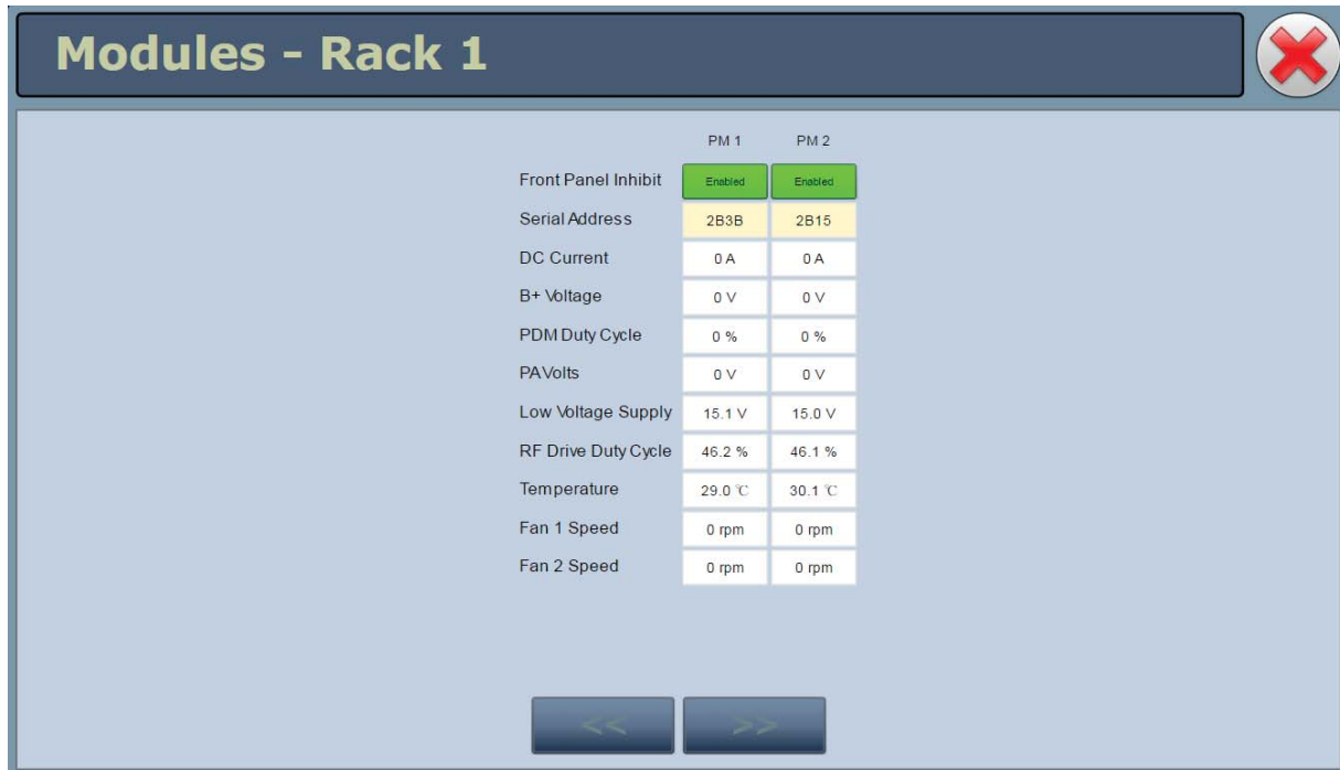
Figure 4.1.6: RF Module Status Screen (all modules)
