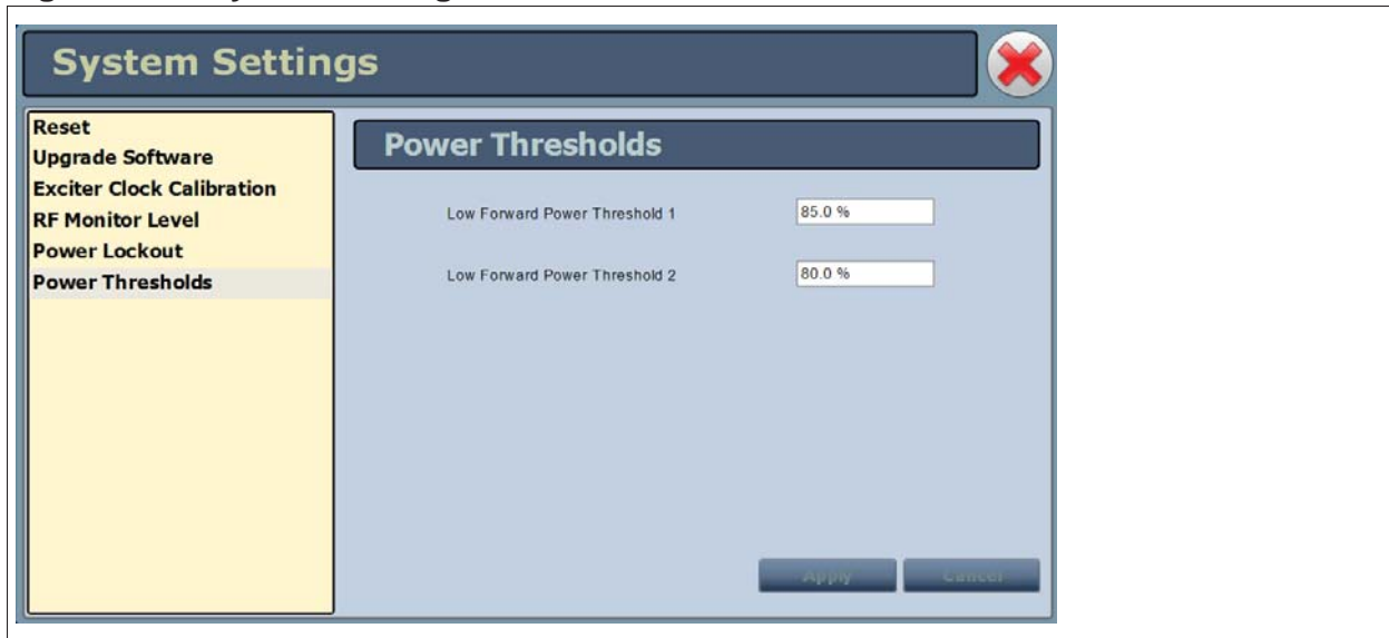
Figure 2.73: System Settings - Power Thresholds
