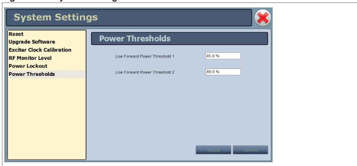
Figure 2.73: System Settings - Power Thresholds
