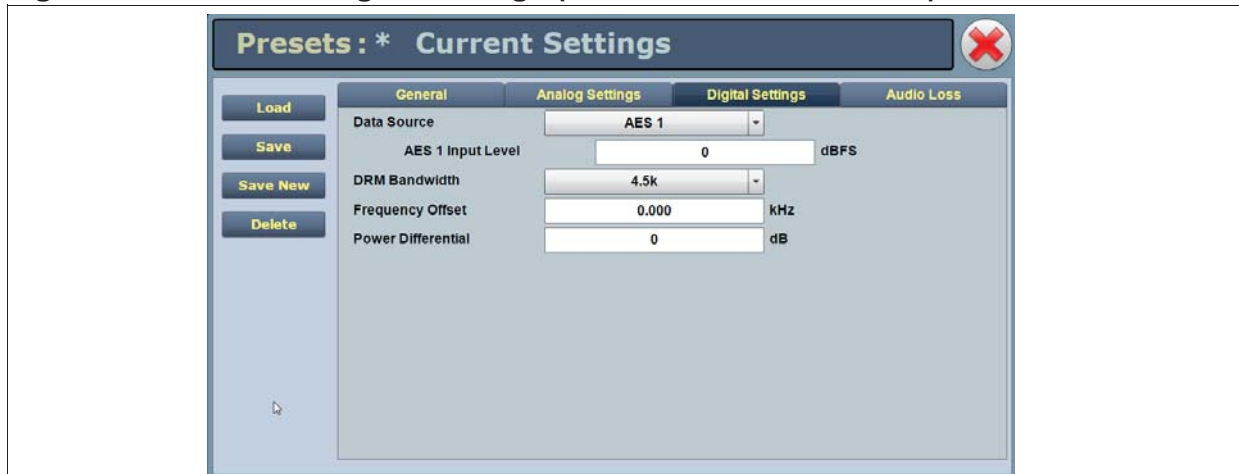
Figure 2.39: Presets - Digital Settings (Overall Mode = DRM+AM)
