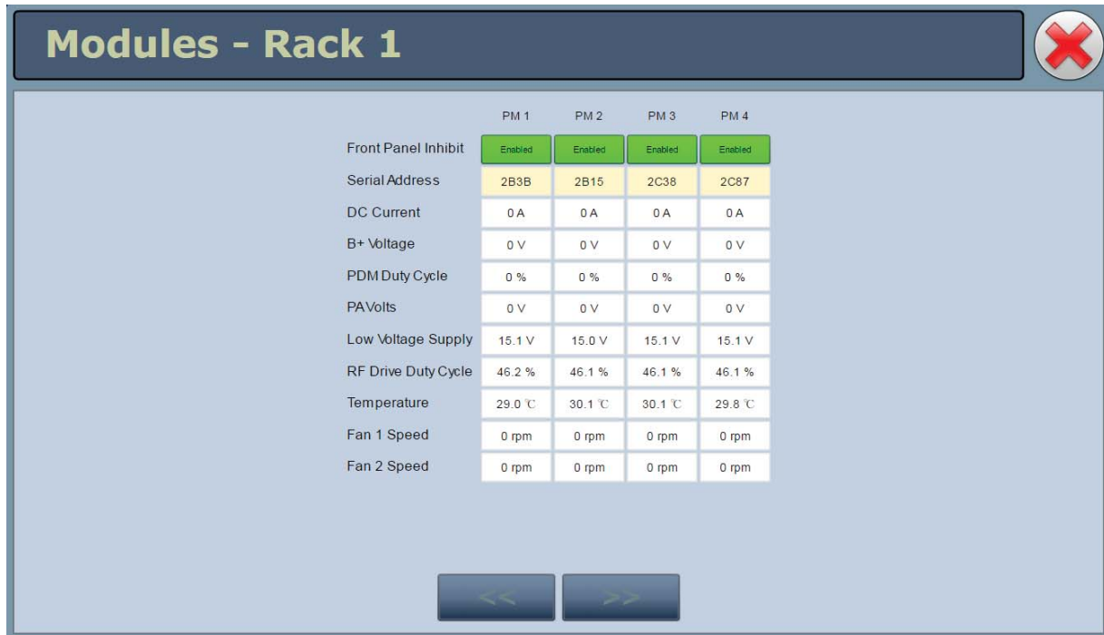
Figure 4.1.6: RF Module Status Screen (all modules)
