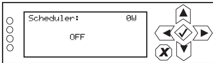
Figure 3.2.158: Enabling/disabling the scheduler - Front Panel
