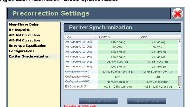
Figure 2.82: Precorrection - Exciter Synchronization
