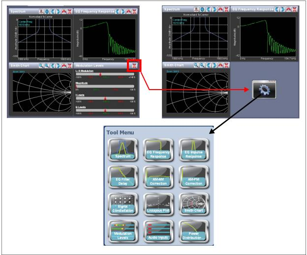
To view the instrument panel options, close an existing panel by pressing **X** (upper-right corner) and then press the "cog" icon to open the *Tool Menu*. Press an icon to display that panel.
