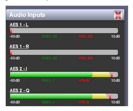
**AUDIO INPUTS.** See Figure 2.26. Bar graphs display the amplitude (in dB) of the audio inputs selected in the preset.
