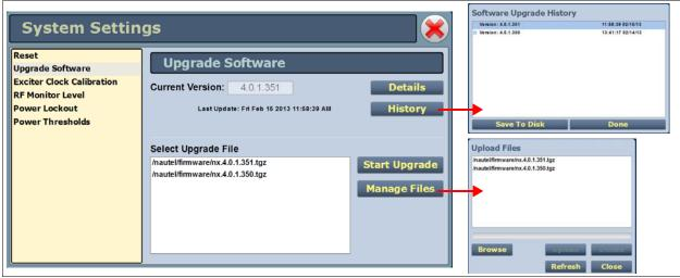
Select the **Upgrade Software** option from the left side of the **System Settings** page to open a related window on the right side of the page. The page consists of the following sections and buttons:
