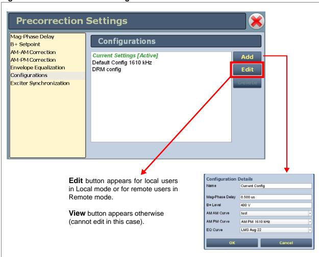
Once a configuration is created, it can be used in a preset. This allows the user to change the precorrection settings based on the operating mode via the preset. Configurations are normally established at the factory, based on customer operating modes, and do not require adjustment.
