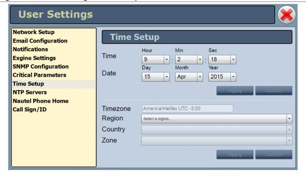
The **Time Setup** option allows users to set the exact time and date information as well as regional and timezone settings for a tranmitter location. All data received from the AUI server (i.e., logs) are timestamped in UTC time. Setting the time zone information allows this timestamp to be adjusted for the user-specific time zone.
