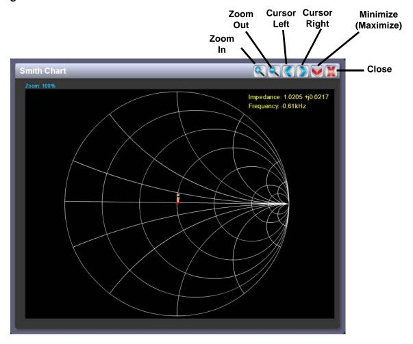
**SMITH CHART.** See Figure 2.24. The Smith Chart allows you to visualize the impedance of the transmitter's load as seen at the combiner, as a function of frequency. The impedance shown on the Smith Chart is normalized to the combiner input impedance. The ideal load is therefore 1 +j0 ohms, which implies a perfect 50-ohm load is being applied to the output of the transmitter.
