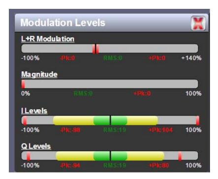
**MODULATION LEVELS.** See Figure 2.25. Bar graphs display the percentage of L+R modulation, PDM (magnitude) and I/Q modulation for the transmitter. I/Q bar graphs will show levels in DRM or IBOC mode only.
