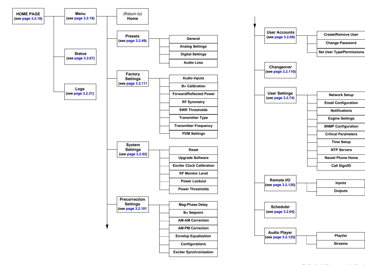
: ][ i fY'&"2: NX Transmitter AUI Flow Diagram
