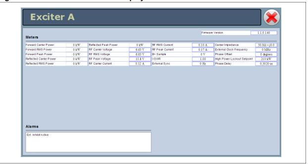
Figure 2.32: Meters - Information Display for Rack 1
