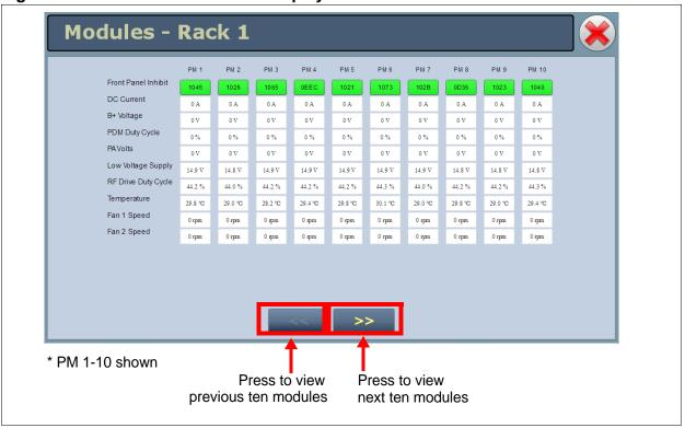
Figure 2.33: Meters - Information Display for Modules - Rack 1
