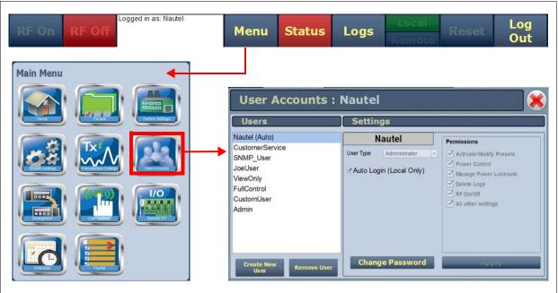
In the *User Accounts* page, users are listed in a panel on the left side of the screen, operations appear along the bottom and settings appear in the center.
