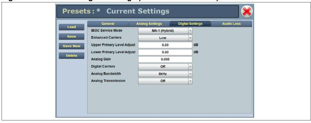
Figure 2.41: Presets - Digital Settings (Overall Mode = IBOC+AM)
