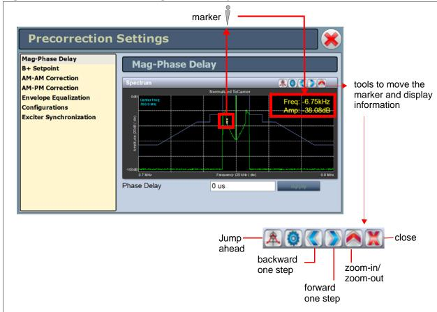
Figure 2.76: Precorrection - Mag-Phase Delay
