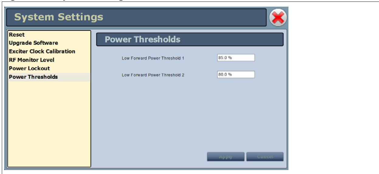
Figure 2.72: System Settings - Power Thresholds
