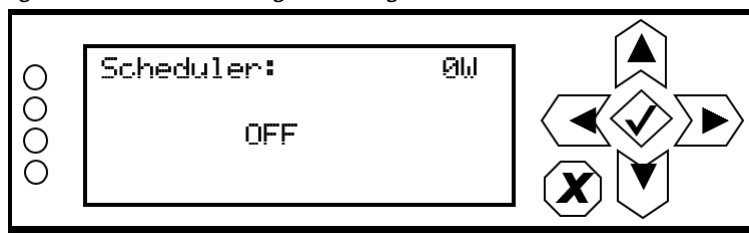
Figure 3.2.159: Enabling/disabling the scheduler - Front Panel
