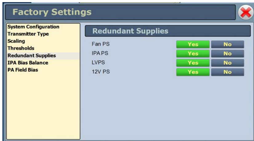
Figure 2.48: Factory Settings - Redundant Supplies
