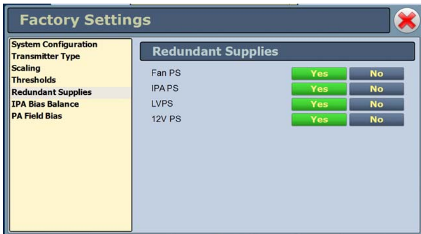
Figure 2.48: Factory Settings - Redundant Supplies
