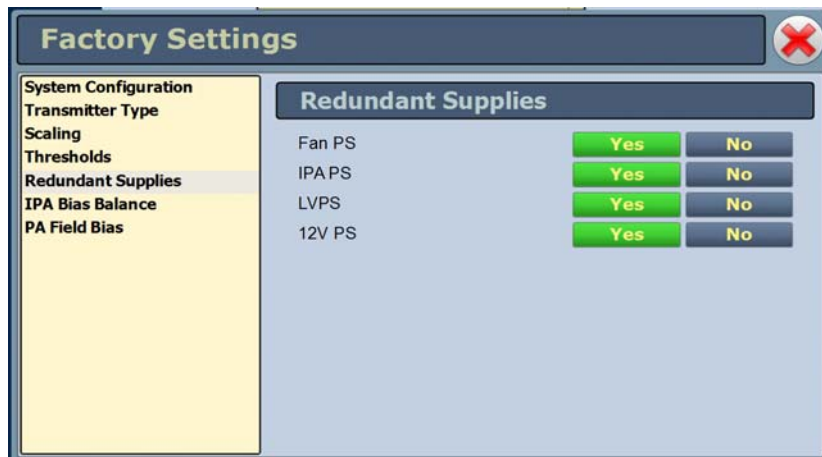
Figure 2.48: Factory Settings - Redundant Supplies
