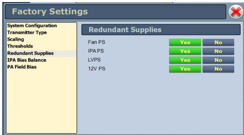
Figure 2.48: Factory Settings - Redundant Supplies
