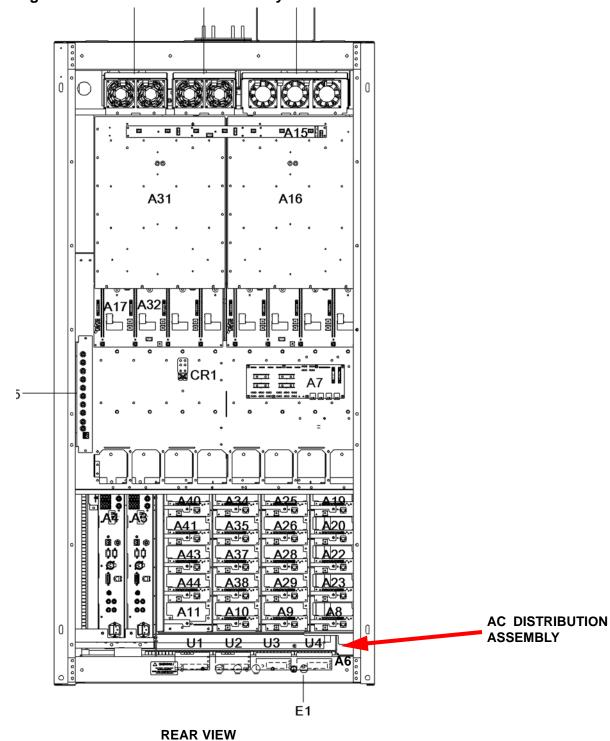
Figure 4.5: Ac Distribution Assembly Location
