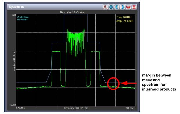
Figure 4.1: Spectrum Analyzer plot on AUI
