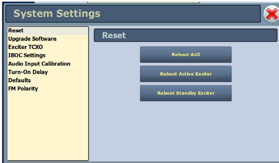
Procedure to reset the AUI or either Exciter:
