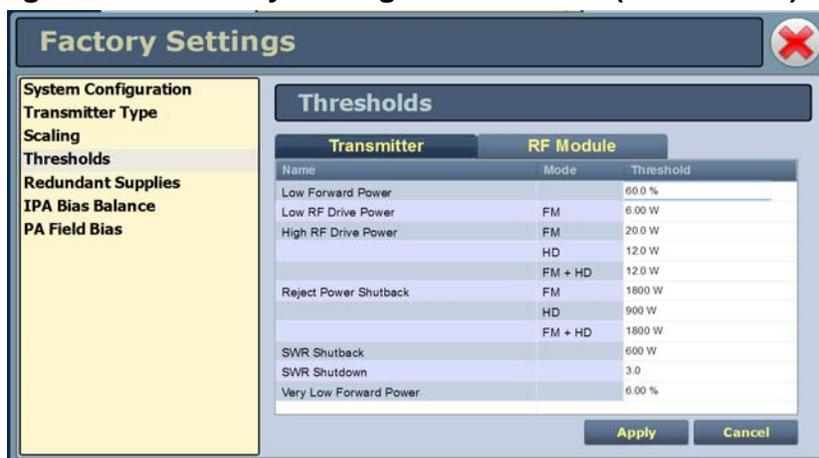
**Figure 2.47: Factory Settings - Thresholds (RF Modules)- Default Values Shown**
