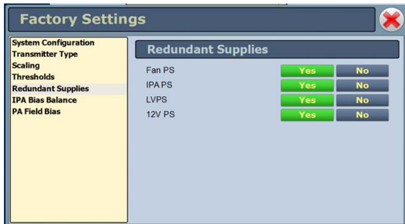
Figure 2.48: Factory Settings - Redundant Supplies
