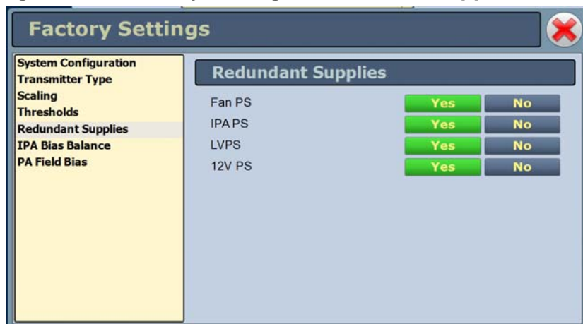
Figure 2.48: Factory Settings - Redundant Supplies
