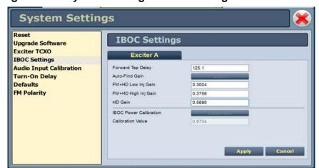
Figure 2.55: System Settings - IBOC Settings
