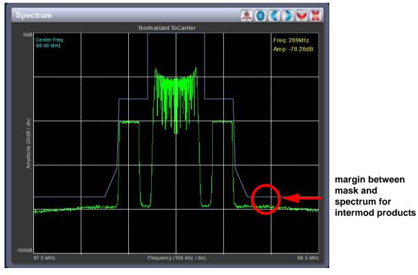
Figure 4.1: Spectrum Analyzer plot on AUI
