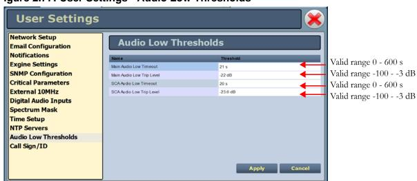
Figure 2.77: User Settings - Audio Low Thresholds
