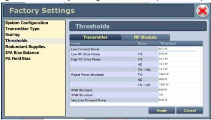
Figure 2.47: Factory Settings - Thresholds (RF Modules)- Default Values Shown
