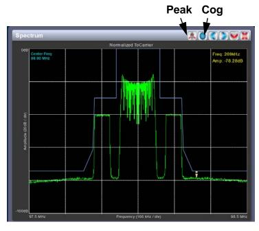
Use the left and right buttons to make fine adjustments.
