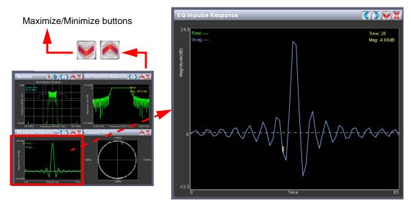
Figure 2.19: Instrument Panel - Expansion Example 2
