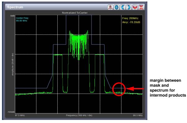
Figure 4.1: Spectrum Analyzer plot on AUI
