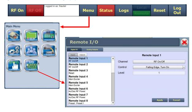
Under the **Digital I/O** tab, press the **Inputs** (see Figure 2.81 on page 2-105) or **Outputs** (see Figure 2.82 on page 2-106) tab to view or edit the configuration of the digital inputs or outputs. Press the **Analog Outputs** tab to configure analog outputs (see on page 2-108).
