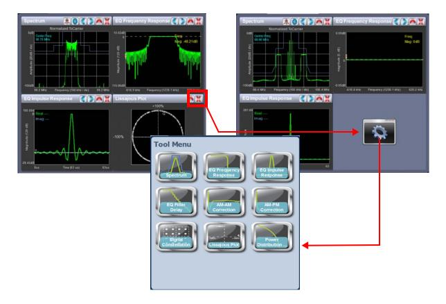
To view the instrument panel options, close an existing panel by pressing X (upper-right corner) and then press the icon in the blank space to open the Tool Menu. Select an icon to display that panel.
