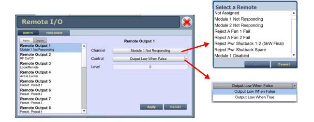
Select the desired digital output (1 through 24) from the list. The **Channel** and **Control** settings for the selected output, as well as the current logic **Level** (1 or 0), are displayed on the right-hand side of the page. You can define the **Channel** and **Control** settings as follows:
