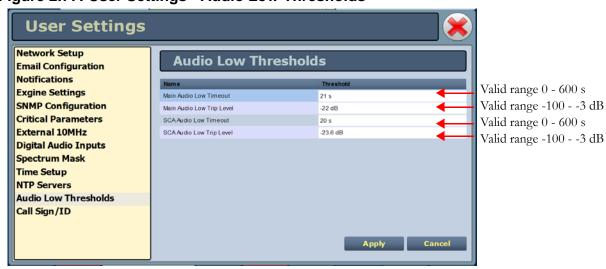
Figure 2.77: User Settings - Audio Low Thresholds
