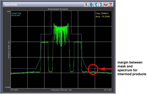
Figure 4.1: Spectrum Analyzer plot on AUI
