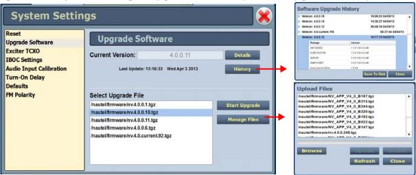
Select the **Upgrade Software** option from the left-side of the **System Settings** page to open a related window on the right-side of the page. The page consists of the following sections and buttons:
