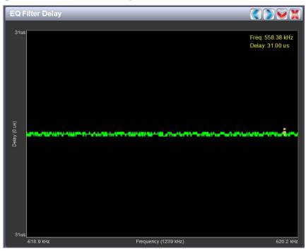
Figure 2.24: EQ Filter Delay
