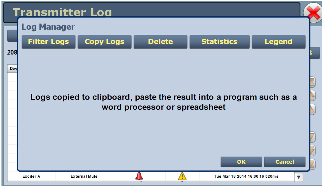
Figure 3.2.14: Log Manager - Copy Logs
