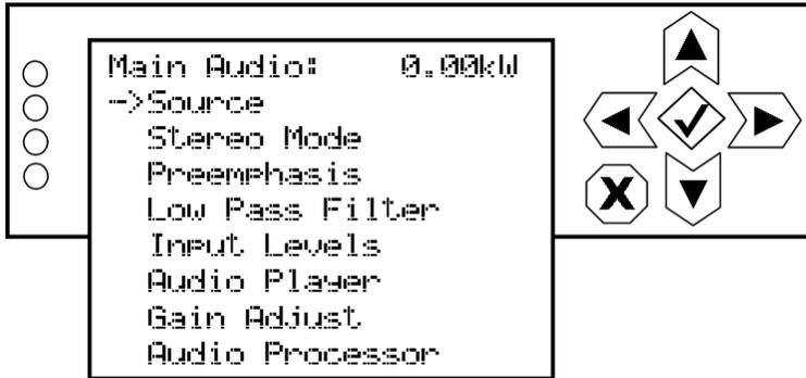
Use the up and down buttons to scroll through the main audio menu options, then press the accept (checkmark) or right arrow button to enter the selected editing screen. [Figure 3.2.49](#) shows the editing screens for the Main Audio menu. Press the cancel (X) button to discard changes and return to the previous menu.
