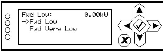
Use the up and down buttons to move the cursor to the desired line item and then press the right button to enable editing. [Figure 3.2.101](#) shows the two editing screens for the Fwd Low menu. Within either of the editing screens, use the up and down buttons to edit the setting. Press the accept (checkmark) button to save the change. Press cancel (X) to discard changes and return to the previous menu.
