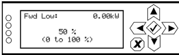
Select a threshold between 0 and 100% (in 0.5% increments), that corresponds to a percentage of rated power. Press the cancel (X) button to discard changes and return to the previous menu. Default setting is 50% (equivalent to 3 dB power reduction).
