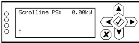
Enter a name. Use the right and left arrows to move the cursor to the desired character. Use the up and down arrows to edit the character, then press the accept (checkmark) button to save the change. Press the cancel (X) button to discard changes and return to the previous menu.
