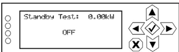
Configures the transmitter to enable (ON) or disable (OFF) the standby exciter's RF power stage to allow testing into a user provided dummy load. When enabled (ON), the exciter will operate at 100 W (ensure the test load is suitably rated). While enabled, auto exciter changeover is disabled (regardless of configuration status). Press the cancel (X) button to discard changes and return to the previous menu.
