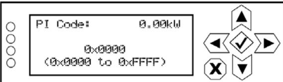
Use the up and down arrows to select a hex value between 0x0000 and 0xFFFF, then press the accept (checkmark) button to save the change. Press the cancel (X) button to discard changes and return to the previous menu. The default hex value is 0x0000.
