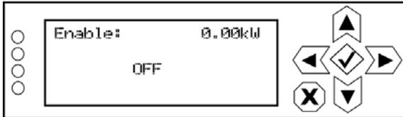
Use the up and down arrows to select ON or OFF, then press the accept (checkmark) button to save the change. Press the cancel (X) button to discard changes and return to the previous menu. Default selection is OFF.
