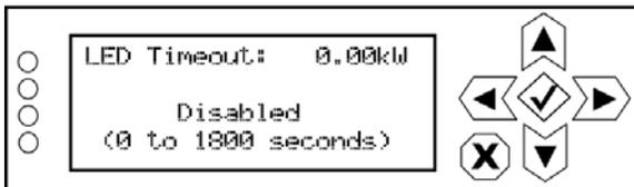
Select disabled (i.e., no timeout) or select a time period between 0 and 1800 seconds (30 minutes) (in 5 s increments). Press the cancel (X) button to discard changes and return to the previous menu. Default setting is 900 s (15 minutes).
