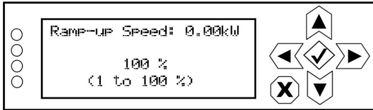
Use the up and down buttons to select a ramp-up speed between 1 and 100% (in 1% increments), noting 100% represents approximately seven seconds (0 W to full power). The default setting is 100%. Press the accept (checkmark) button to save the change. Press X to abort the change and return to the previous menu.
