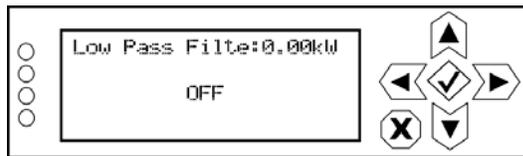
Use the up and down buttons to toggle between ON or OFF, then press the accept (checkmark) button to save the change. Press the cancel (X) button to discard changes and return to the previous menu. Default setting is OFF.
