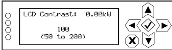
Select a value between 50 (lighter contrast) and 200 (darker contrast) (in increments of 5). Press the cancel (X) button to discard changes and return to the previous menu. Default setting is 100.
