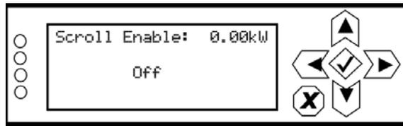
Use the up and down arrows to select Off, Fast or Slow, then press the accept (checkmark) button to save the change. Press the cancel (X) button to discard changes and return to the previous menu. The default selection is Off.
