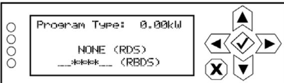
Use the up and down arrows to select the program type from the various options, then press the accept (checkmark) button to save the change. Press the cancel (X) button to discard changes and return to the previous menu. The default selection is NONE.
