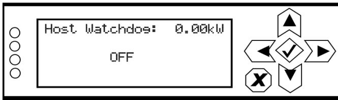
Use the up and down buttons to toggle between Enabled and Disabled. Press the accept (checkmark) button to save the change. Press cancel (X) to discard changes and return to the previous menu.
