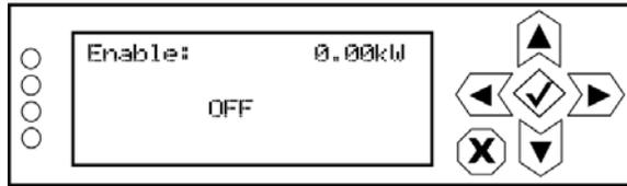
Determines whether the audio loss feature is used. Use the up and down arrows to select ON (enable) or OFF (disable), then press the accept (checkmark) button to save the change. Press the cancel (X) button to discard changes and return to the previous menu. Default selection is OFF.
