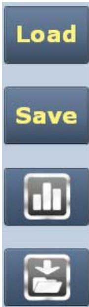
When you first enter the Audio Processor page, the current preset is displayed. If the current preset is not the preset you want to work with, press the Load button to call up a window containing a list of alternate presets. Presets that display an 'F' are factory presets that cannot be modified. Presets that display a 'U' are user presets that can be modified.
