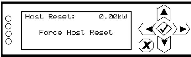
Use the up and down buttons to toggle between Force Host Reset and Cancel. Press the accept (checkmark) button to save the change. If a reset is selected, it will occur immediately. Select Cancel or press X to abort the reset and return to the previous menu.
