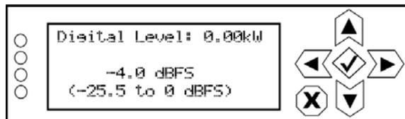
Use the up and down buttons to select a level between -25.5 and 0 dBFS (in 0.1 dBFS increments) then press the accept (checkmark) button to save the change. Press the cancel (X) button to discard changes and return to the previous menu. Default level is -4.0 dBFS.
