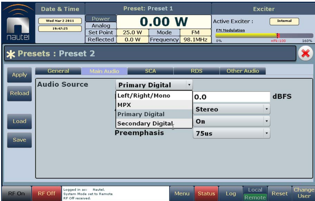
Figure 3.4.2: Backup Preset Main Audio Screen
