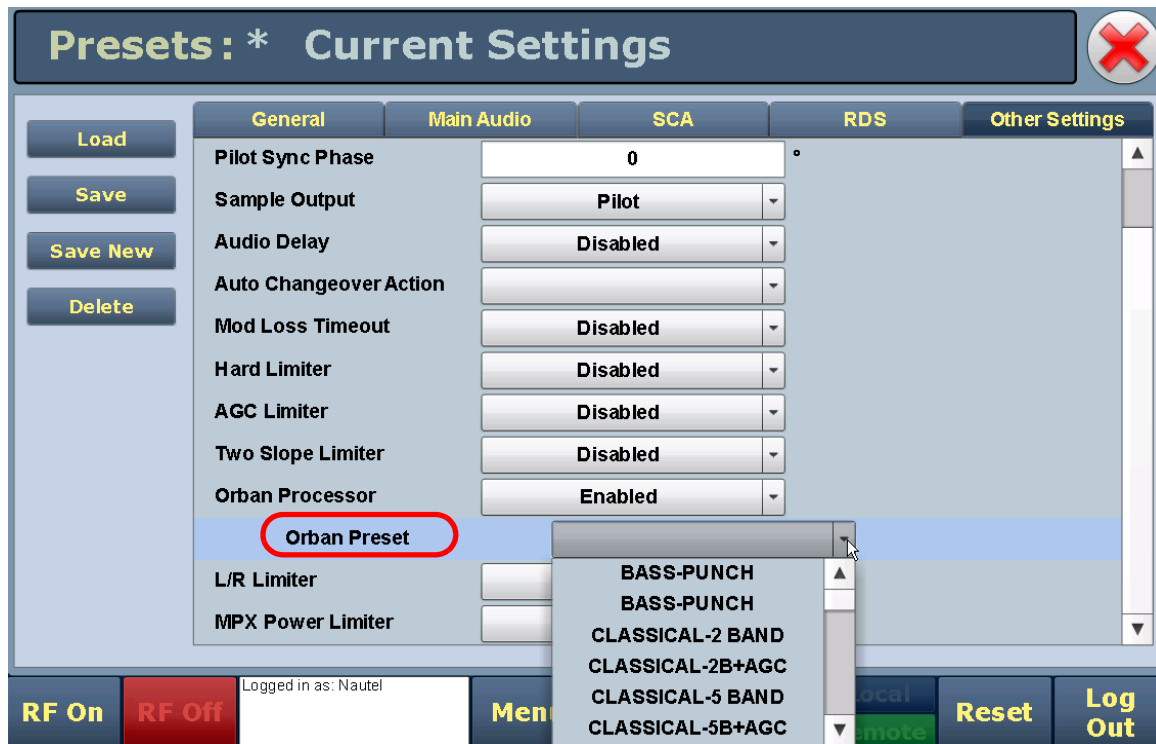
Figure 3.2.155: Selecting an Orban Preset - Remote AUI
