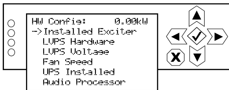
Figure 3.2.118: HW Config Menu
