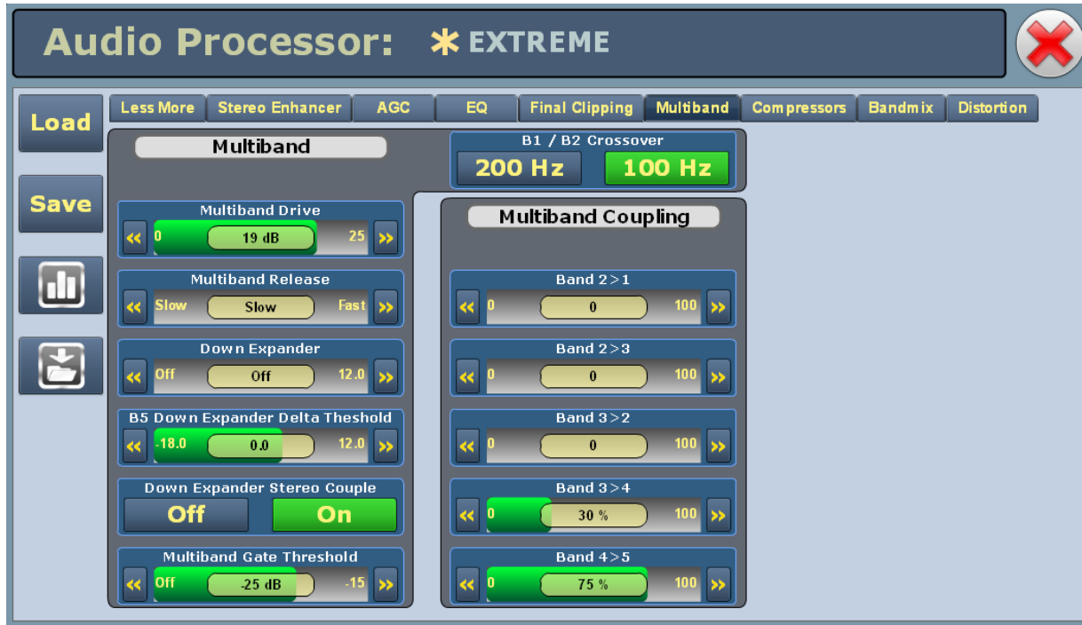
Figure 3.2.163: Audio Processor Menu - Multiband tab
