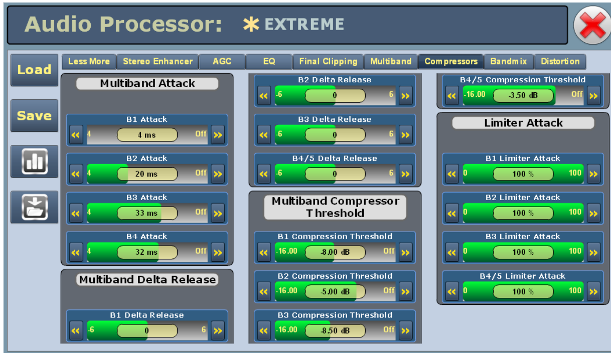
Figure 3.2.164: Audio Processor Menu - Compressors tab
