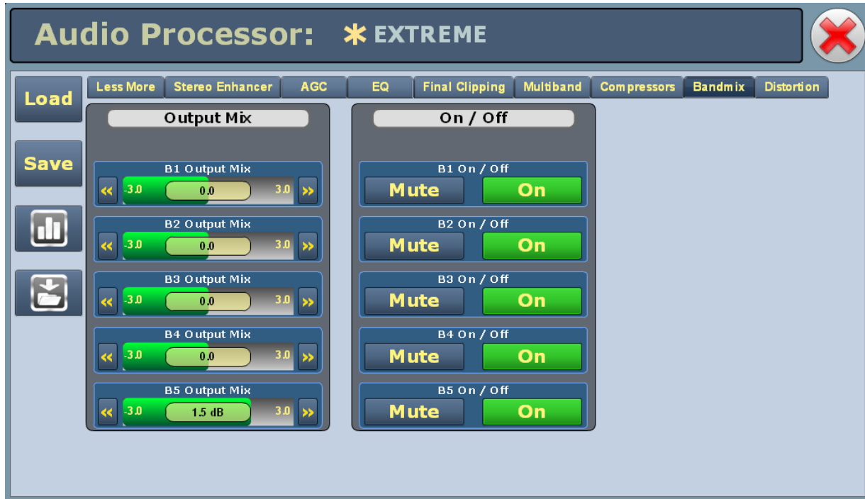
Figure 3.2.165: Audio Processor Menu - Bandmix tab
