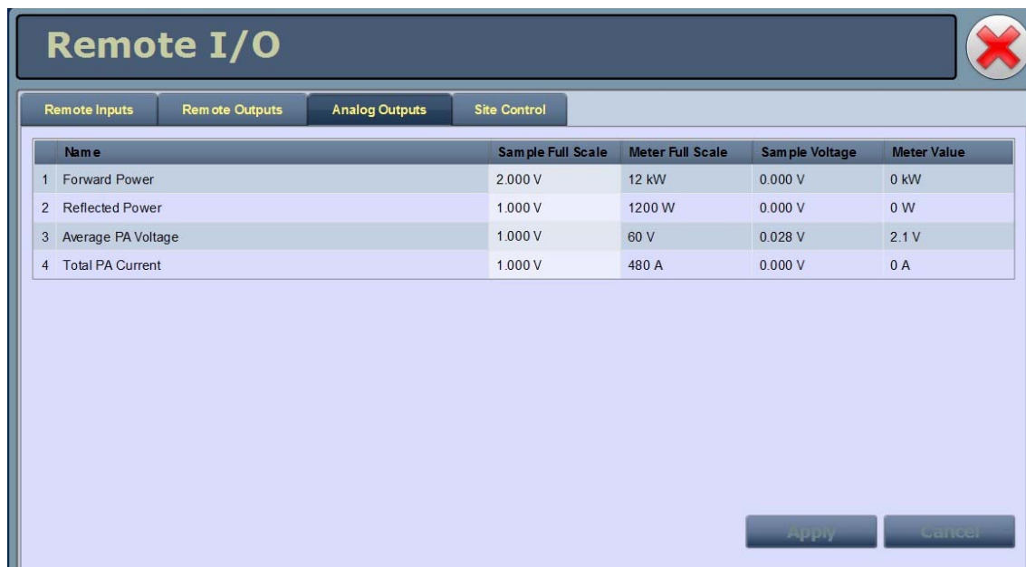
Figure 3.2.136: Remote I/O Page - Analog Outputs tab selected
