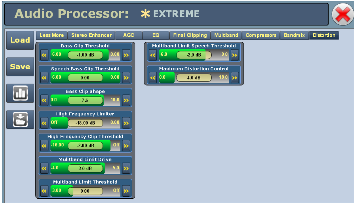
Figure 3.2.166: Audio Processor Menu - Distortion tab
