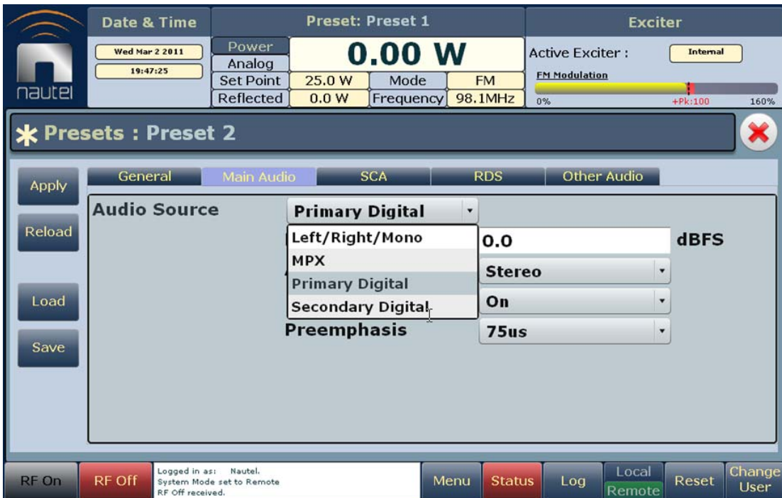
Figure 3.4.2: Backup Preset Main Audio Screen
