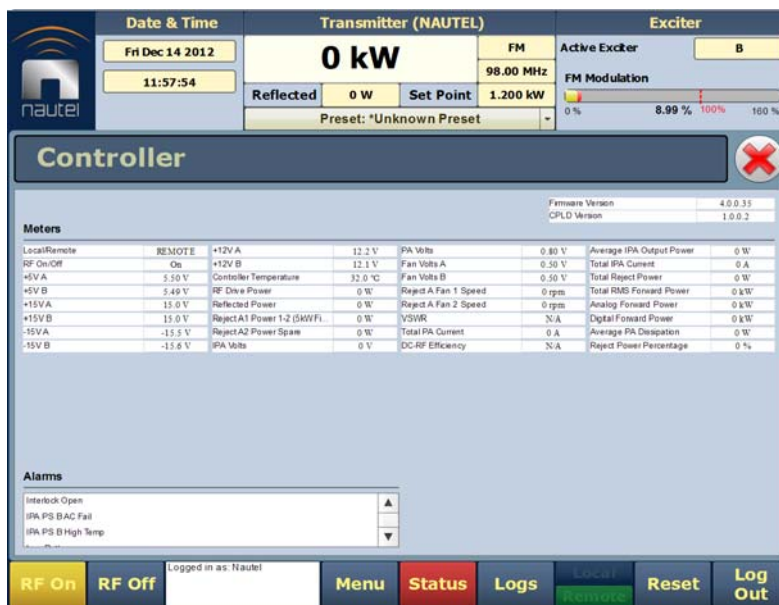
Figure 3.2.33: Meters - Information (Device type Controller shown)
