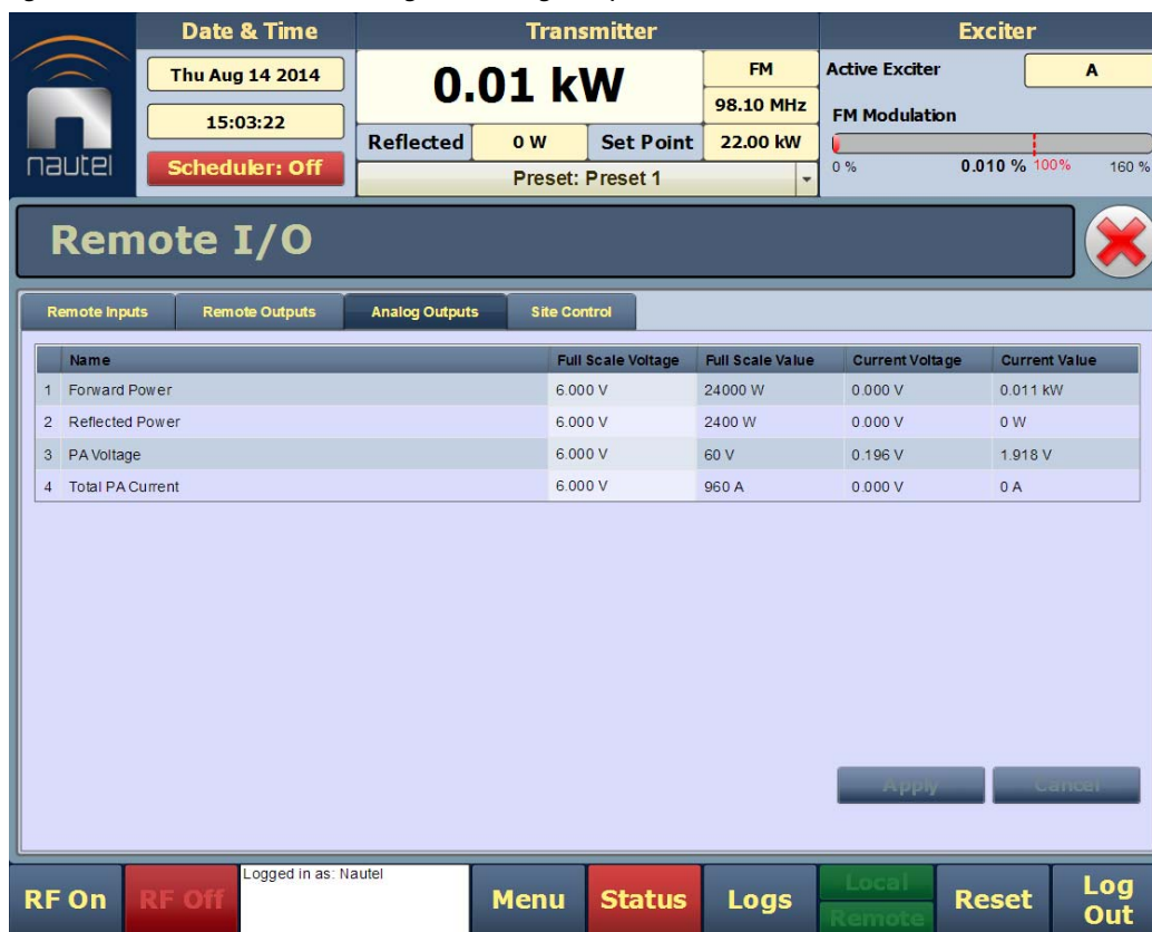
Figure 3.2.136: Remote I/O Page - Analog Outputs tab selected
