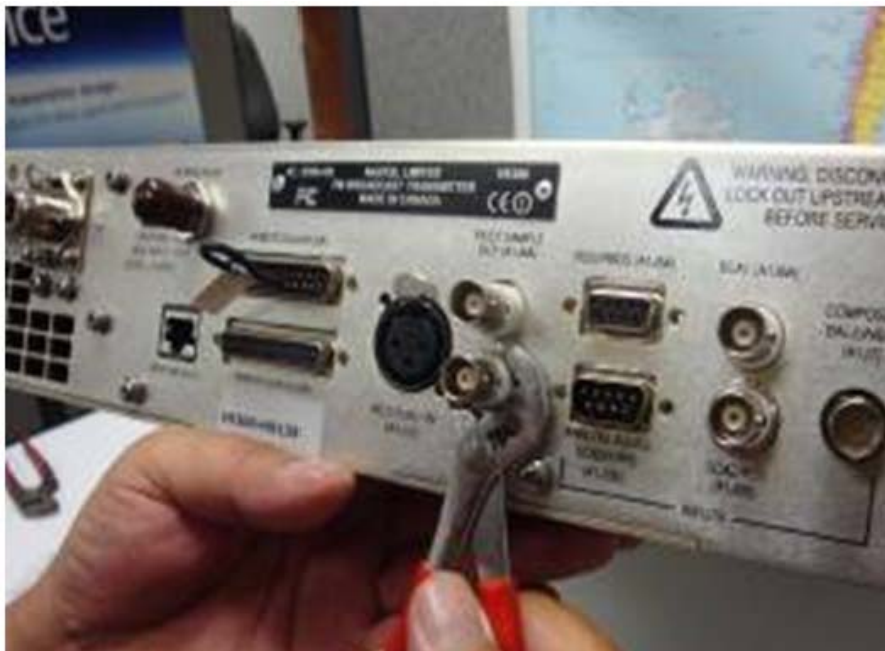
Figure 4.1.29: Loosening the BNC connector's locking ring
