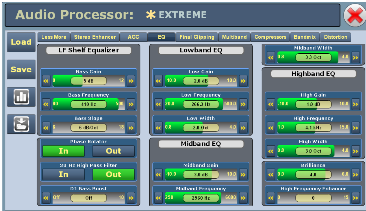
Figure 3.2.180: Audio Processor Menu - EQ tab
