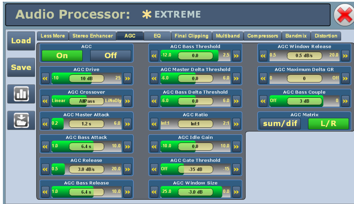
Figure 3.2.179: Audio Processor Menu - AGC tab
