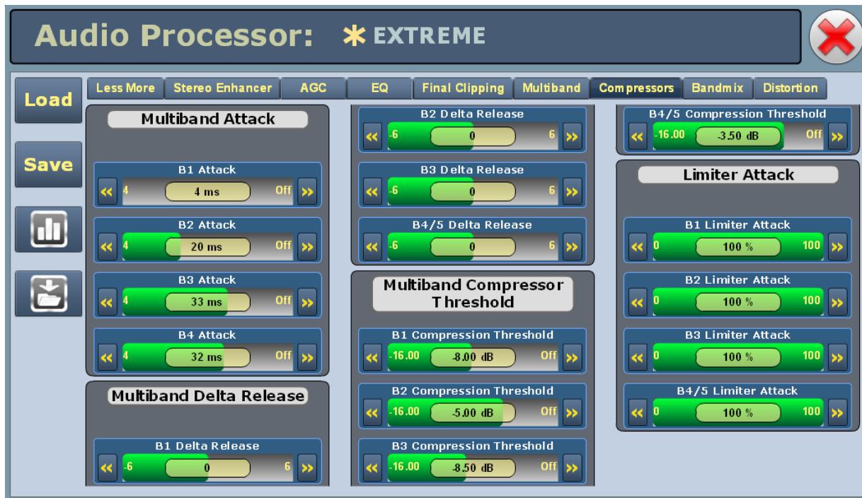
Figure 3.2.183: Audio Processor Menu - Compressors tab
