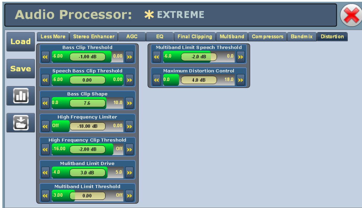
Figure 3.2.185: Audio Processor Menu - Distortion tab
