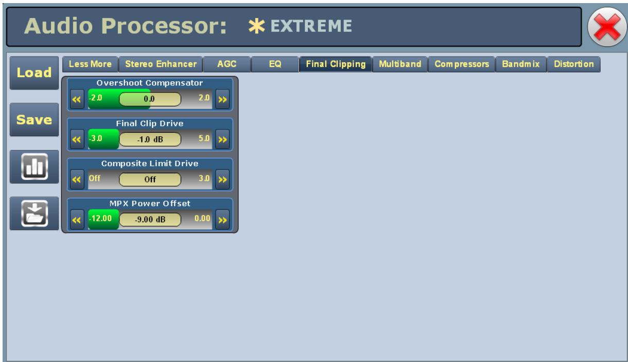
Figure 3.2.181: Audio Processor Menu - Final Clipping tab
