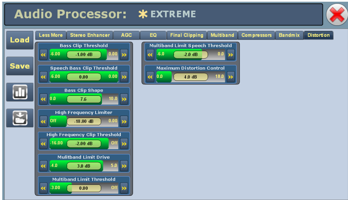
Figure 3.2.185: Audio Processor Menu - Distortion tab
