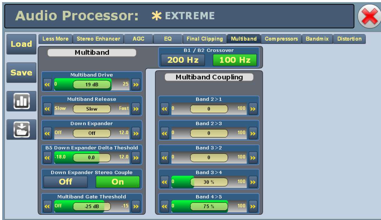
Figure 3.2.182: Audio Processor Menu - Multiband tab
