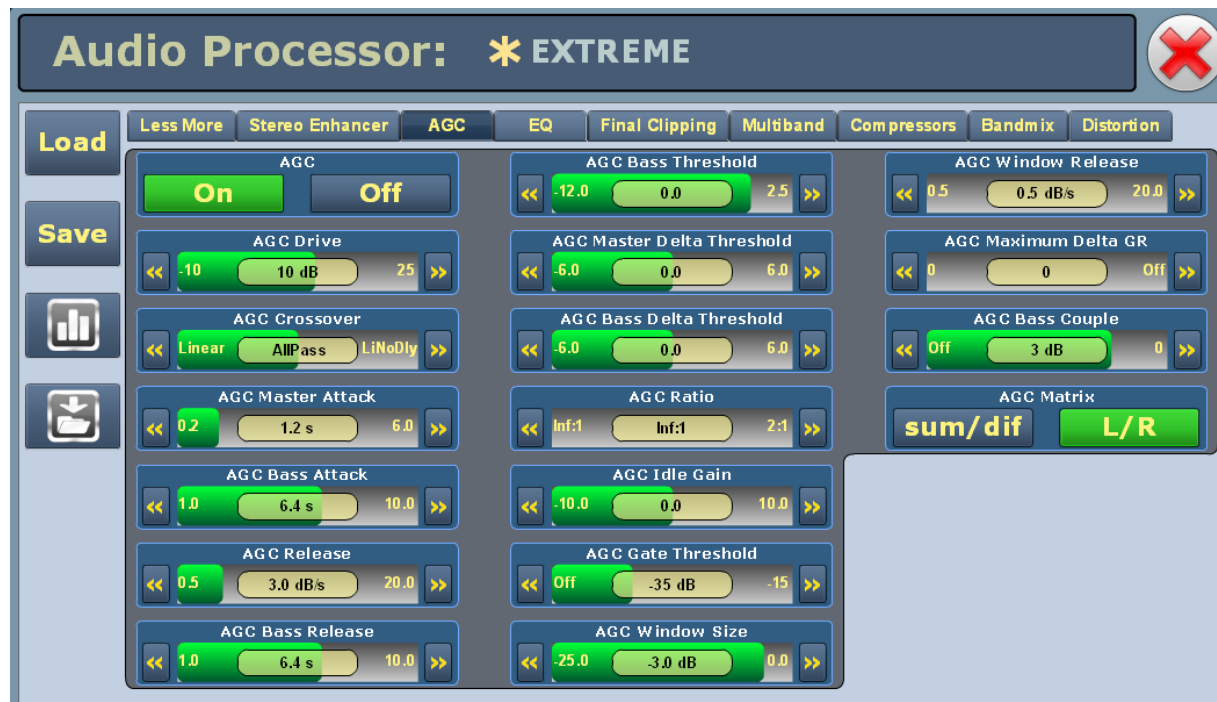
Figure 3.2.179: Audio Processor Menu - AGC tab
