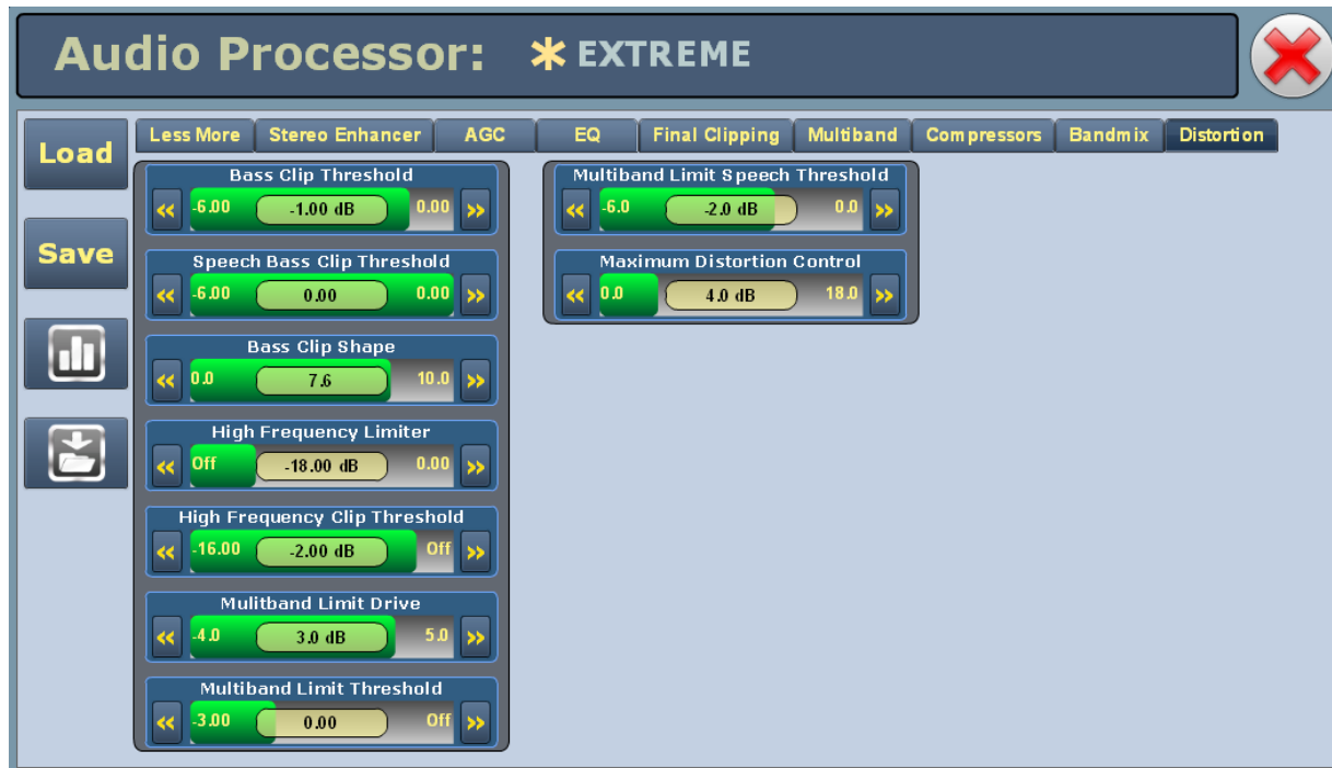
Figure 3.2.185: Audio Processor Menu - Distortion tab
