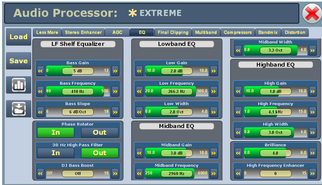
Figure 3.2.180: Audio Processor Menu - EQ tab
