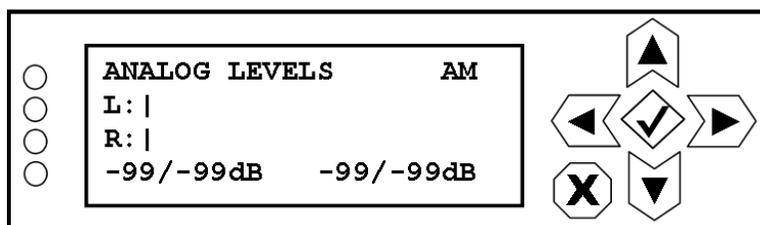
L: bar display of the left channel level (average/peak shown in dBFS at bottom, left of screen)
