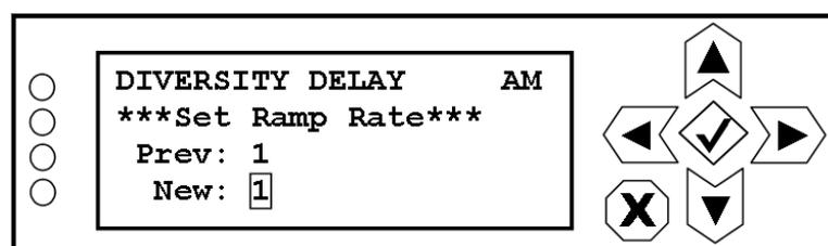
Use the up and down buttons to increase or decrease the value of the ramp rate. The ramp rate is defined as a multiple of the diversity delay. See [“Overview” on page 1-1](#) for additional information.
