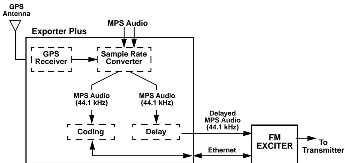
Figure 1.2: Exporter Plus in an AM HD radio system
