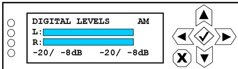
L: bar display of the left channel level (average/peak shown in dB at bottom, left of screen)
