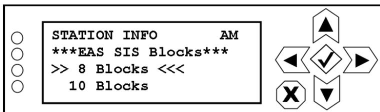
Use the up and down buttons to select the desired number of blocks (8, 10, 11 or 12). Press the accept or cancel button to enter the Save/Cancel screen (see [Figure 8.4 on page 8-5](#)). Save or cancel as desired.
