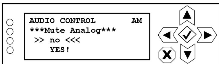
Use the up and down buttons to highlight YES! or no. Press the accept or cancel button to enter the Save/Cancel screen (see [Figure 8.4 on page 8-5](#)). Save or cancel as desired. Selecting YES! mutes the analog audio input.
