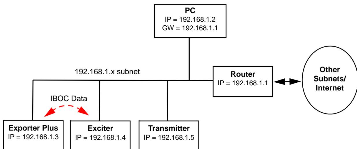
In this case, only one Ethernet port (ETH0) on the Exporter Plus requires configuration and IP forwarding is not required. If access to devices on other subnets is not necessary, then gateway address configuration is also not required.
