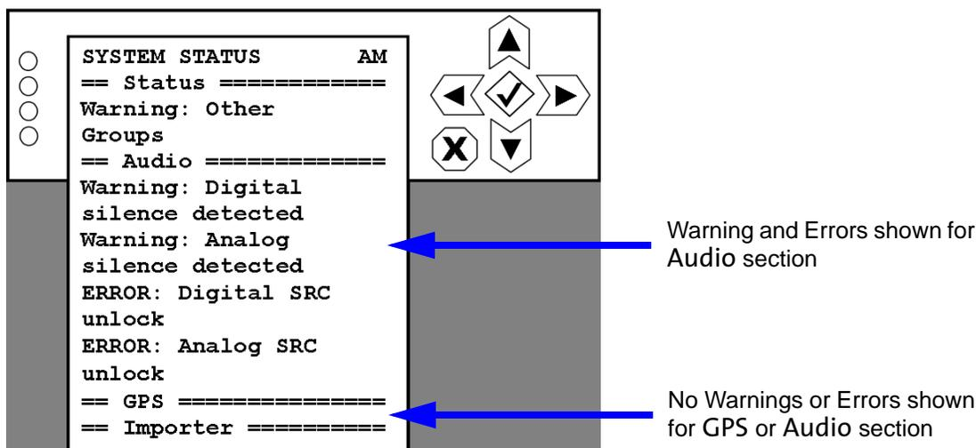
This screen displays applicable alarm details associated with the four LEDs (Status, Audio, GPS and Importer). Alarm details are preceded by “Warning” or “ERROR”. See [Table 8.4](#) for a list of possible alarm occurrences. If no text is displayed, there are no alarms or warnings present.
