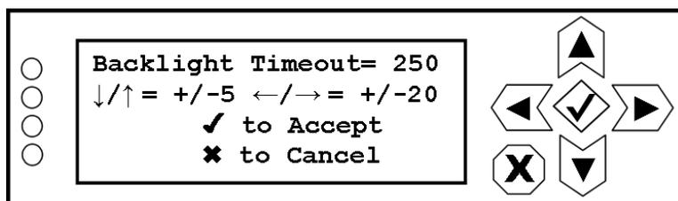
The current backlight timeout (in seconds) is displayed on the top line.
