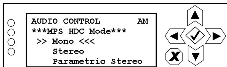
Use the up and down buttons to highlight the desired mode (Mono, Stereo or Parametric Stereo). Mono or Parametric Stereo is recommended when the Exporter Plus is in AM mode with enhanced carriers disabled. Stereo is recommended for all other modes. Press the accept or cancel button to enter the Save/Cancel screen (see [Figure 8.4 on page 8-5](#)). Save or cancel as desired.
