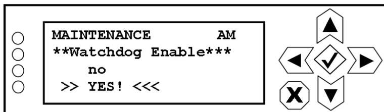
Use the up and down buttons to highlight Yes or No. Selecting Yes enables the watchdog timer. Press the accept or cancel button to enter the Save/Cancel screen (see [Figure 8.4 on page 8-5](#)). Save or cancel as desired.
