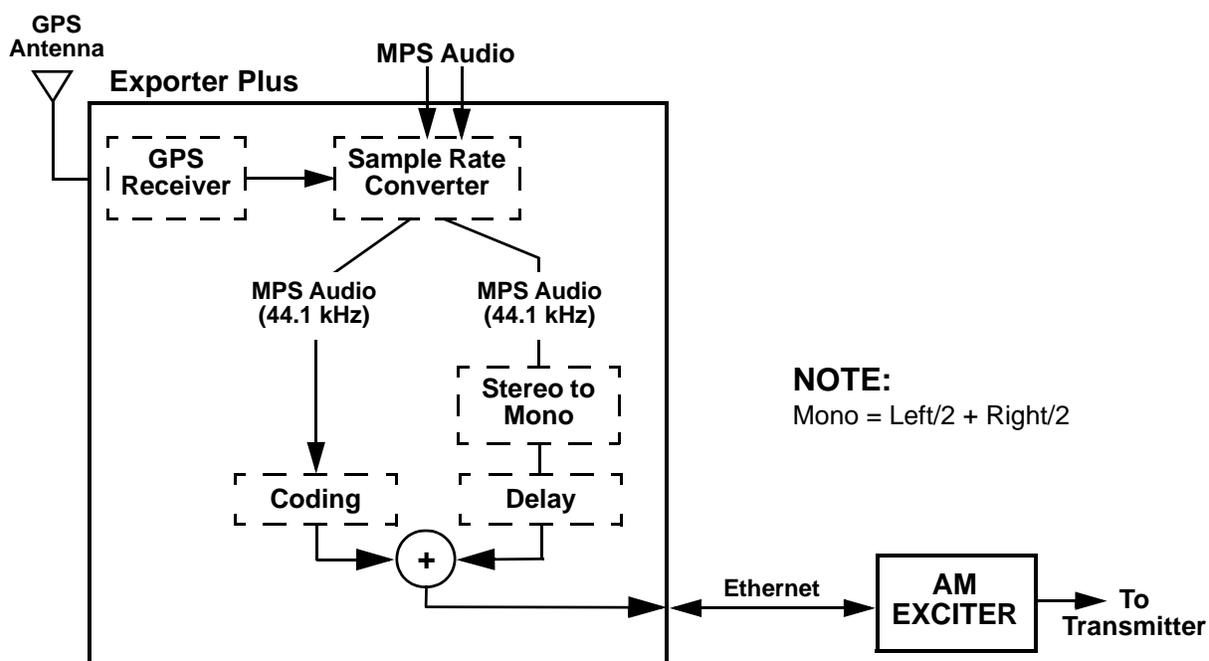
**Note:** Other common system components, such as Ethernet switches and audio processors, are not shown. They are described later. [Figure 1.1](#) and [Figure 1.2](#) are based on a combined IBOC system.
