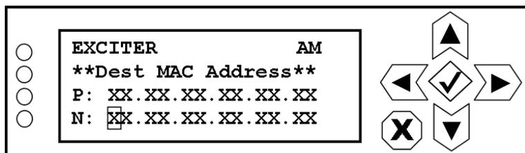
Use the right and left buttons to highlight the desired digit in the new address, then use the up and down buttons to change the value of the highlighted digit. Press the accept or cancel button to enter the Save/Cancel screen (see [Figure 8.4 on page 8-5](#)). Save or cancel as desired.
