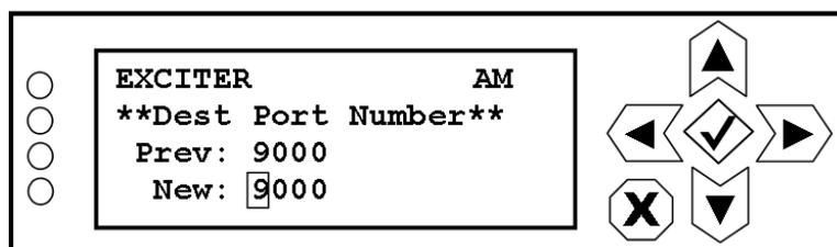
Use the right and left buttons to highlight the desired digit in the new port number, then use the up and down buttons to increase or decrease the value of the highlighted digit. Press the accept or cancel button to enter the Save/Cancel screen (see [Figure 8.4 on page 8-5](#)). Save or cancel as desired.
