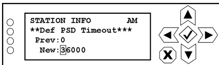
Use the right and left buttons to highlight the desired digit in the new default PSD timeout value (in minutes), then use the up and down buttons to increase or decrease the value as desired. Setting this value to 0 will disable the PSD Fault Timeout alarm. The maximum setting is 36,000 seconds (10 hours). Press the accept or cancel button to enter the Save/Cancel screen (see [Figure 8.4 on page 8-5](#)). Save or cancel as desired.
