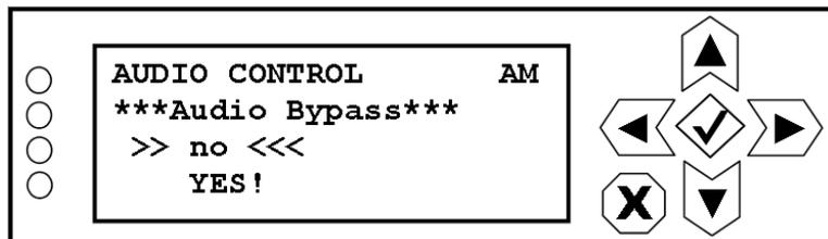
Use the up and down buttons to highlight YES! or no. Press the accept or cancel button to enter the Save/Cancel screen (see [Figure 8.4 on page 8-5](#)). Save or cancel as desired. Selecting YES! bypasses the analog audio and connects the audio input directly to the analog output.
