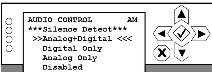
Use the up and down buttons to highlight the desired input type to enable (Analog+Digital, Digital Only or Analog Only) or disable (Disabled). Press the accept or cancel button to enter the Save/Cancel screen (see [Figure 8.4 on page 8-5](#)). Save or cancel as desired. Selecting Disabled mutes associated alarms when no inputs are being applied.
