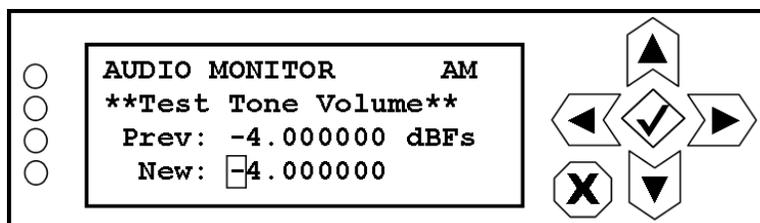
Use the right and left buttons to highlight the desired digit in the new test tone volume value, then use the up and down buttons to increase or decrease the value (in dBFs) of the highlighted digit. Press the accept or cancel button to enter the Save/Cancel screen (see [Figure 8.4 on page 8-5](#)). Save or cancel as desired.
