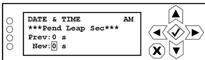
Use the right and left buttons to highlight the desired digit in the pending leap seconds, then use the up and down buttons to change the digit as desired. Press the accept or cancel button to enter the Save/Cancel screen (see [Figure 8.4 on page 8-5](#)). Save or cancel as desired.
