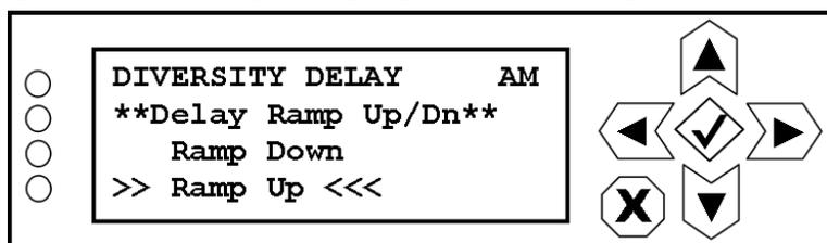
Use the up and down buttons to highlight the desired ramping type (Ramp Up or Ramp Down). Press the accept or cancel button to enter the Save/Cancel screen (see [Figure 8.4 on page 8-5](#)). Save or cancel as desired.
