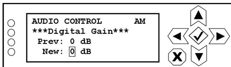
Use the up and down buttons to increase and decrease the new digital gain setting (between -8 and +7 dB). Press the accept or cancel button to enter the Save/Cancel screen (see [Figure 8.4](#) on page 8-5). Save or cancel as desired.
