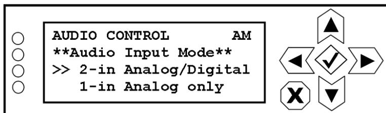
Use the up and down buttons to highlight the desired mode (2-in Analog/Digital or 1-in Analog only). Press the accept or cancel button to enter the Save/Cancel screen (see [Figure 8.4 on page 8-5](#)). Save or cancel as desired.
