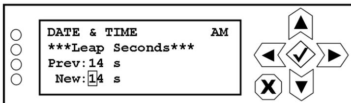
Use the right and left buttons to highlight the desired digit in the leap seconds, then use the up and down buttons to change the digit as desired. Press the accept or cancel button to enter the Save/Cancel screen (see [Figure 8.4 on page 8-5](#)). Save or cancel as desired.
