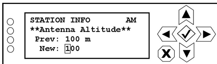
Use the right and left buttons to highlight the desired digit in the new antenna altitude value, then use the up and down buttons to increase or decrease the value as desired. Press the accept or cancel button to enter the Save/Cancel screen (see [Figure 8.4 on page 8-5](#)). Save or cancel as desired.
