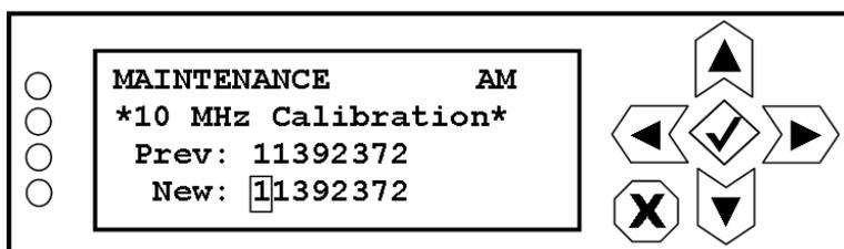
Use the right and left buttons to highlight the desired digit in the new 10 MHz calibration value, then use the up and down buttons to increase or decrease the value of the highlighted digit. You can set the calibration value between 0 and 268431360. Press the accept or cancel button to enter the Save/Cancel screen (see [Figure 8.4 on page 8-5](#)). Save or cancel as desired.
