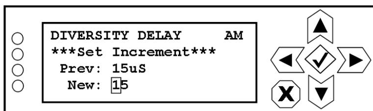
Use the right and left buttons to highlight the desired digit in the new increment value, then use the up and down buttons to increase or decrease the value of the highlighted digit. You can set the delay increment between 0 and 999 microseconds. Press the accept or cancel button to enter the Save/Cancel screen (see [Figure 8.4 on page 8-5](#)). Save or cancel as desired.
