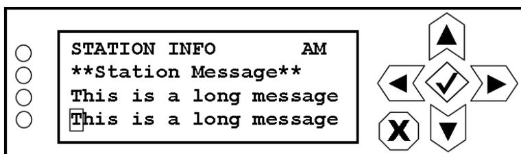
Use the right and left buttons to highlight the desired character in the new station message, then use the up and down buttons to change the character as desired. The station message can be up to 190 characters in length. Press the accept or cancel button to enter the Save/Cancel screen (see [Figure 8.4 on page 8-5](#)). Save or cancel as desired.
