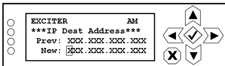
Use the right and left buttons to highlight the desired digit in the new address, then use the up and down buttons to increase or decrease the value of the highlighted digit. Press the accept or cancel button to enter the Save/Cancel screen (see [Figure 8.4 on page 8-5](#)). Save or cancel as desired.
