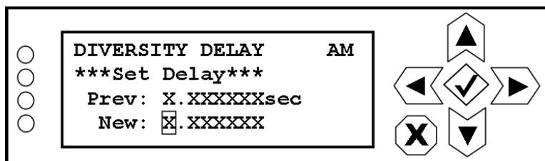
Use the right and left buttons to highlight the desired digit in the new delay value, then use the up and down buttons to increase or decrease the value of the highlighted digit. You can set the diversity delay between 0 and 20 seconds. Press the accept or cancel button to enter the Save/Cancel screen (see [Figure 8.4 on page 8-5](#)). Save or cancel as desired.
