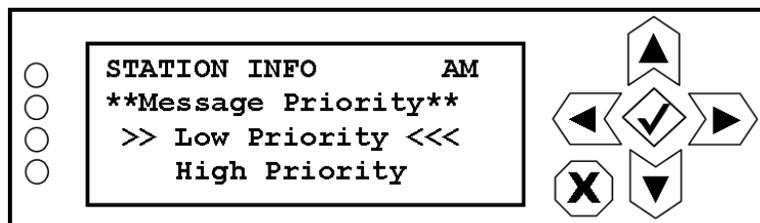
Use the up and down buttons to highlight Low Priority or High Priority. Selecting High Priority makes your station message more noticeable on certain receivers. For example, the receiver may precede a high priority message with an 'ALERT' indication. Press the accept or cancel button to enter the Save/Cancel screen (see [Figure 8.4 on page 8-5](#)). Save or cancel as desired.
