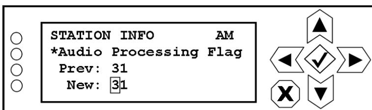
Use the right and left buttons to highlight the desired digit in the new audio processing flag value, then use the up and down buttons to increase or decrease the value as desired. Press the accept or cancel button to enter the Save/Cancel screen (see [Figure 8.4 on page 8-5](#)). Save or cancel as desired.
