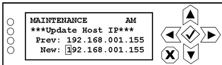
Use the right and left buttons to highlight the desired digit in the new address, then use the up and down buttons to increase or decrease the value of the highlighted digit. Press the accept or cancel button to enter the Save/Cancel screen (see [Figure 8.4 on page 8-5](#)). Save or cancel as desired.
