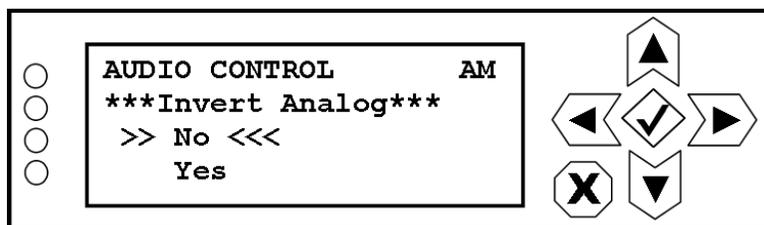
Use the up and down buttons to highlight Yes or No. Press the accept or cancel button to enter the Save/Cancel screen (see [Figure 8.4 on page 8-5](#)). Save or cancel as desired. Selecting Yes inverts the phase of the analog audio input.
