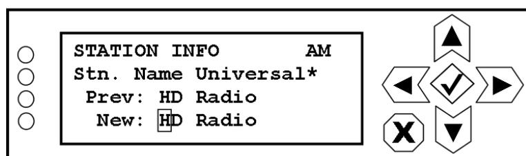
Use the right and left buttons to highlight the desired character in the new universal station name, then use the up and down buttons to change the character as desired. The universal station name is intended for internal applications only and can be up to 12 characters in length. Press the accept or cancel button to enter the Save/Cancel screen (see [Figure 8.4 on page 8-5](#)). Save or cancel as desired.
