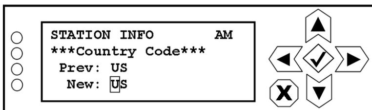
Use the right and left buttons to highlight the desired character in the new country code, then use the up and down buttons to change the character as desired. Use the appropriate 2-character country codes specified by ISO 3166-1-alpha-2. Typically, this code will be factory set. Press the accept or cancel button to enter the Save/Cancel screen (see [Figure 8.4 on page 8-5](#)). Save or cancel as desired.
