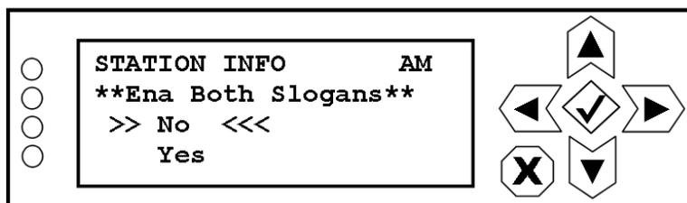
Use the up and down buttons to highlight Yes or No. Selecting Yes enables both slogans. Press the accept or cancel button to enter the Save/Cancel screen (see [Figure 8.4 on page 8-5](#)). Save or cancel as desired.
