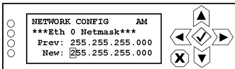
Use the right and left buttons to highlight the desired digit in the new address, then use the up and down buttons to change the value of the highlighted digit. Press the accept or cancel button to enter the Save/Cancel screen (see [Figure 8.4 on page 8-5](#)). Save or cancel as desired.
