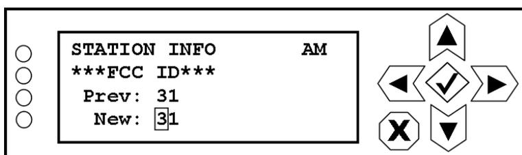
Use the right and left buttons to highlight the desired digit in the new FCC ID value, then use the up and down buttons to increase or decrease the value as desired. Typically, this value will be provided to you by the FCC. Press the accept or cancel button to enter the Save/Cancel screen (see [Figure 8.4 on page 8-5](#)). Save or cancel as desired.
