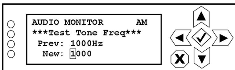
Use the right and left buttons to highlight the desired digit in the new test tone frequency, then use the up and down buttons to increase or decrease the value of the highlighted digit. You can adjust the test tone frequency between 50 Hz and 10,000 Hz. Press the accept or cancel button to enter the Save/Cancel screen (see [Figure 8.4 on page 8-5](#)). Save or cancel as desired.
