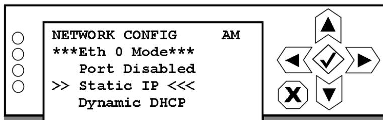
Use the up and down buttons to highlight the desired mode (Port Disabled, Static IP or Dynamic DHCP). Press the accept or cancel button to enter the Save/Cancel screen (see [Figure 8.4 on page 8-5](#)). Save or cancel as desired.
