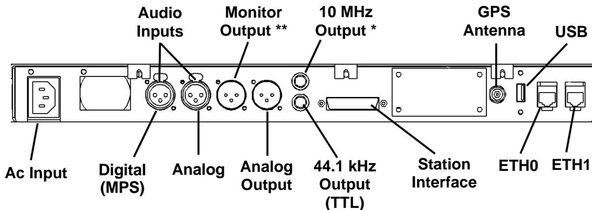
\* - Not typically used. Normally, the 10 MHz is provided via ETH0.
