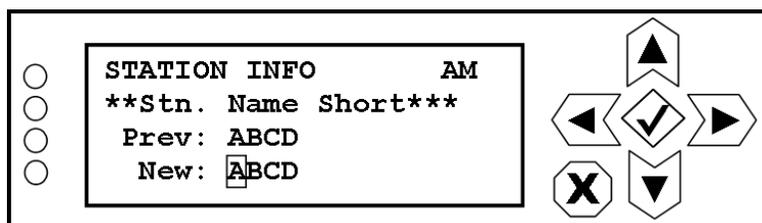
Use the right and left buttons to highlight the desired character in the new short station name, then use the up and down buttons to change the character as desired. Only standard, 4-character call signs are supported. The short station name will be displayed on the top line of the MAIN MENU of the UI. Press the accept or cancel button to enter the Save/Cancel screen (see [Figure 8.4 on page 8-5](#)). Save or cancel as desired.
