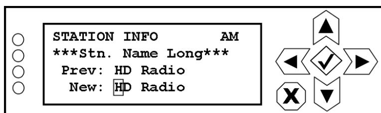
Use the right and left buttons to highlight the desired character in the new long station name, then use the up and down buttons to to change the character as desired. The long station name can be up to 56 characters in length. Press the accept or cancel button to enter the Save/Cancel screen (see [Figure 8.4 on page 8-5](#)). Save or cancel as desired.
