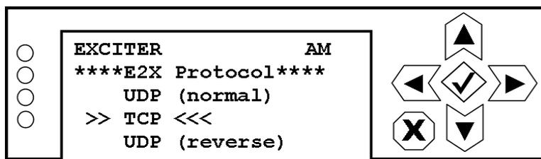
Use the up and down buttons to highlight UDP (normal), TCP or UDP (reverse). Select UDP (reverse) only as advised by Nautel. Press the accept or cancel button to enter the Save/Cancel screen (see [Figure 8.4 on page 8-5](#)). Save or cancel as desired.
