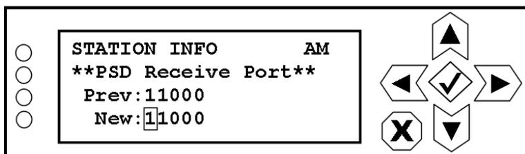
Use the right and left buttons to highlight the desired digit in the new PSD receive port value, then use the up and down buttons to increase or decrease the value as desired. Press the accept or cancel button to enter the Save/Cancel screen (see [Figure 8.4](#) on page 8-5). Save or cancel as desired.
