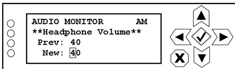
Use the right and left buttons to highlight the desired digit in the new headphone volume value, then use the up and down buttons to increase or decrease the value of the highlighted digit. You can adjust the volume between 0 and 100%. Press the accept or cancel button to enter the Save/Cancel screen (see [Figure 8.4 on page 8-5](#)). Save or cancel as desired.
