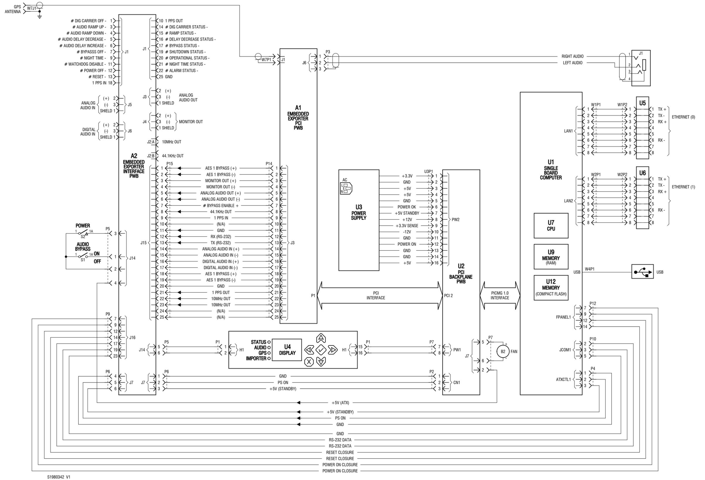
Figure 10-10: Electrical Schematic - Exporter Plus (NAE97E to NAE97K)
