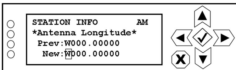
Use the right and left buttons to highlight the desired N (north), S (south) or numeric character in the new latitude coordinate, then use the up and down buttons to change the character as desired. Press the accept or cancel button to enter the Save/Cancel screen (see [Figure 8.4 on page 8-5](#)). Save or cancel as desired.
