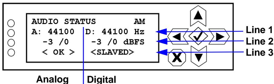
Line 1: Displays lock status for analog and digital audio
