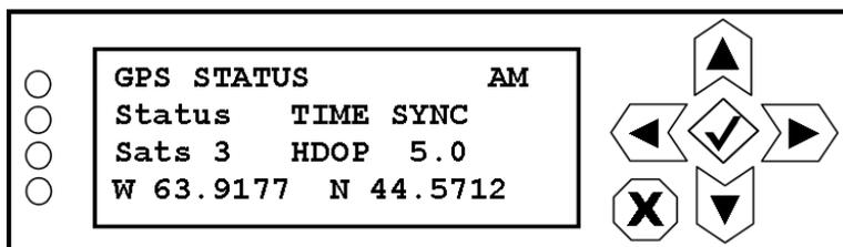
Frequency lock (TIME SYNC displayed) should be assured if the number of detected satellites (Sats) by the GPS receiver is three or more and if the HDOP value is 4 or less. These values will change as satellites move, but generally, if the antenna has a reasonably clear view of the sky, then the values should be at least as good as described above.
