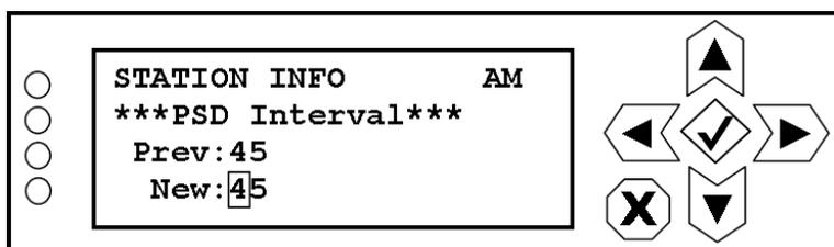
Use the right and left buttons to highlight the desired digit in the new PSD interval value, then use the up and down buttons to increase or decrease the value as desired. Press the accept or cancel button to enter the Save/Cancel screen (see [Figure 8.4 on page 8-5](#)). Save or cancel as desired.
