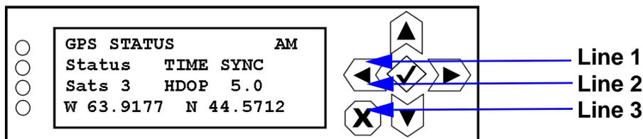
Status: GPS ACQUIRE (no satellites detected), PLL ALIGN (occurs briefly, if 1 PPS OK), PLL UNLOCKED (pulling in), TIME SYNC (locked) or HOLDOVER (coasting; there was a GPS dropout, and the Exporter Plus is now using the internal 10 MHz).
