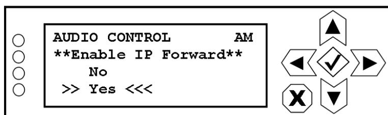
Use the up and down buttons to highlight Yes or no. Press the accept or cancel button to enter the Save/Cancel screen (see [Figure 8.4 on page 8-5](#)). Save or cancel as desired. Selecting Yes enables IP forwarding.
