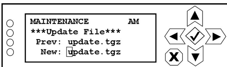
Use the right and left buttons to highlight the desired character in the new update file name, then use the up and down buttons to change the character as desired. Press the accept or cancel button to enter the Save/Cancel screen (see [Figure 8.4 on page 8-5](#)). Save or cancel as desired.
