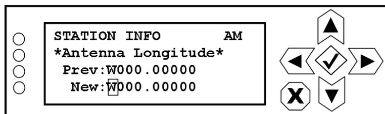
Use the right and left buttons to highlight the desired E (east), W (west) or numeric character in the new longitude coordinate, then use the up and down buttons to change the character as desired. Press the accept or cancel button to enter the Save/Cancel screen (see [Figure 8.4](#) on page 8-5). Save or cancel as desired.
