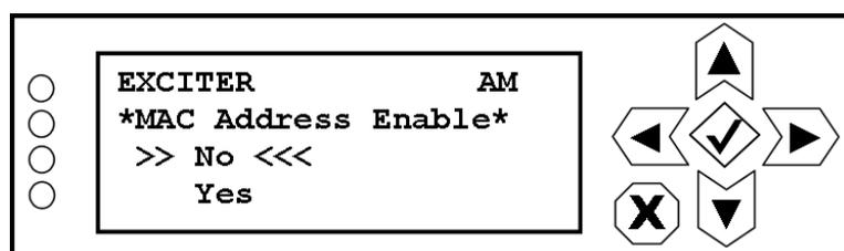
Use the up and down buttons to highlight YES! or no. Press the accept or cancel button to enter the Save/Cancel screen (see [Figure 8.4 on page 8-5](#)). Save or cancel as desired. Selecting YES! enables communication with the previously set destination MAC address [Setting destination MAC address on page 8-23](#).
