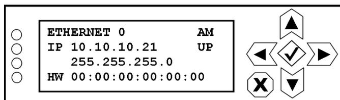
IP: IP address established in [“Setting Ethernet 0 or 1 IP address”](#) on page 8-26. The line below the IP address is the netmask established in [“Setting Ethernet 0 or 1 netmask”](#) on page 8-26.
