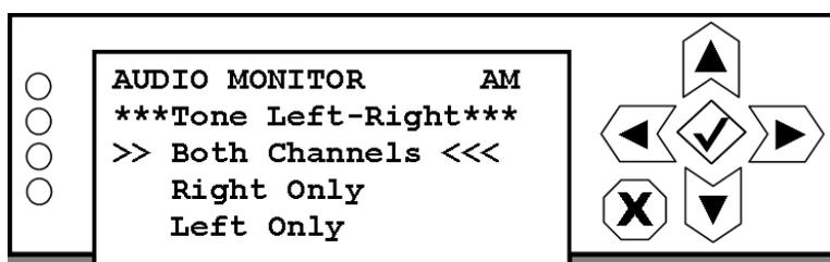
Use the up and down buttons to highlight the desired channel content (Both Channels (L+R), Right Only or Left Only). Press the accept or cancel button to enter the Save/Cancel screen (see [Figure 8.4 on page 8-5](#)). Save or cancel as desired.
