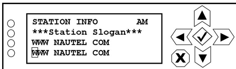
Use the right and left buttons to highlight the desired character in the new slogan, then use the up and down buttons to change the character as desired. The station slogan can be up to 96 characters in length. Press the accept or cancel button to enter the Save/Cancel screen (see [Figure 8.4 on page 8-5](#)). Save or cancel as desired.
