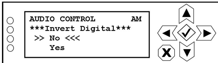
Use the up and down buttons to highlight Yes or No. Press the accept or cancel button to enter the Save/Cancel screen (see [Figure 8.4 on page 8-5](#)). Save or cancel as desired. Selecting Yes inverts the phase of the digital audio input.
