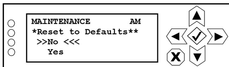
Use the up and down buttons to highlight Yes or No. Selecting Yes enables the reset to defaults, after which you must initiate a restart of the Exporter Plus. Press the accept or cancel button to enter the Save/Cancel screen (see [Figure 8.4 on page 8-5](#)). Save or cancel as desired.
