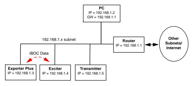
In this case, only one Ethernet port (ETHO) on the Exporter Plus requires configuration and IP forwarding is not required. If access to devices on other subnets is not necessary, then gateway address configuration is also not required.
