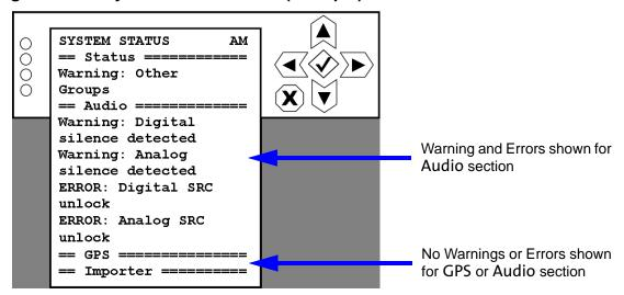
This screen displays applicable alarm details associated with the four LEDs (Status, Audio, GPS and Importer). Alarm details are preceded by "Warning" or "ERROR". See Table 8.4 for a list of possible alarm occurrences. If no text is displayed, there are no alarms or warnings present.
