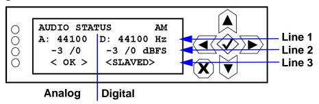
Line 1: Displays lock status for analog and digital audio
