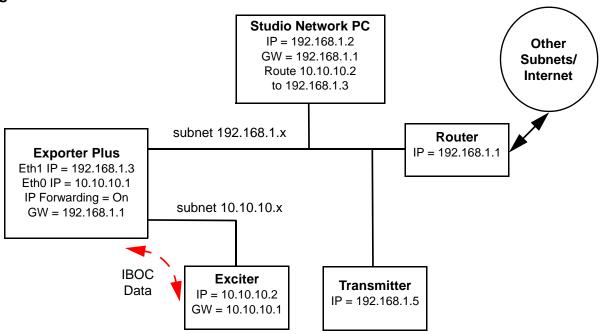
A user on the Studio Network PC will want the ability to browse both the Internet (192.168.1.x subnet) and equipment on the 10.10.10.x subnet. In order to do this the Studio Network PC needs several gateways - one for the Internet router and one for the 10.10.10.x subnet. Typical PC configuration allows for a single gateway, however it is possible to modify the PC routing table to assign gateway addresses to specific IP addresses.
