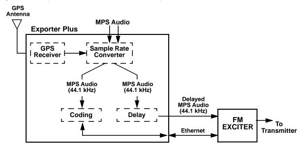
Figure 1.2: Exporter Plus in an AM HD radio system
