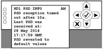
Example of a PSD timeout with time stamp of last PSD received
