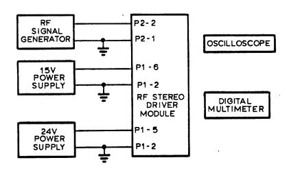
Figure 1 Test Setup for NAPE20 Stereo RF Driver Module
