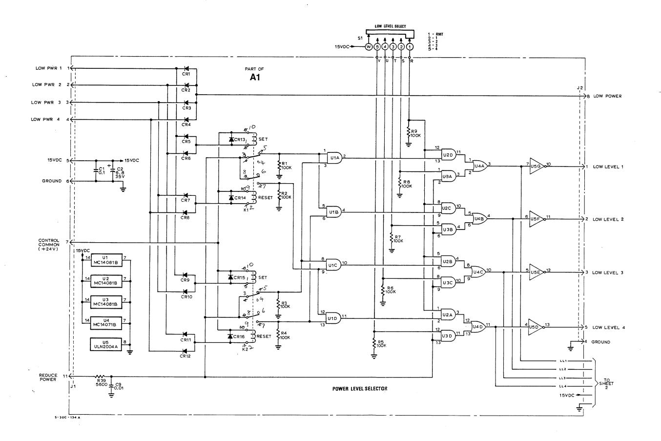
Figure FO-2 Electrical Schematic-NAPC19 Five-Level Power Trim Assembly (Sheet 1 of 2)
