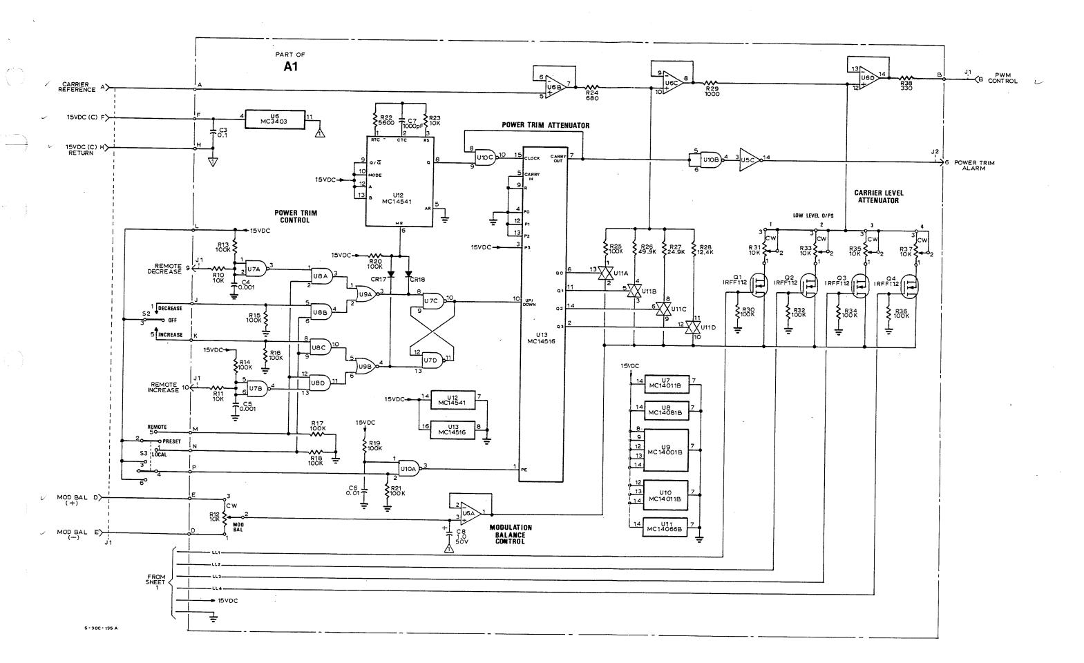
Figure FO-3 Electrical Schematic-NAPC19 Five-Level Power Trim Assembly (Sheet 2 of 2)
