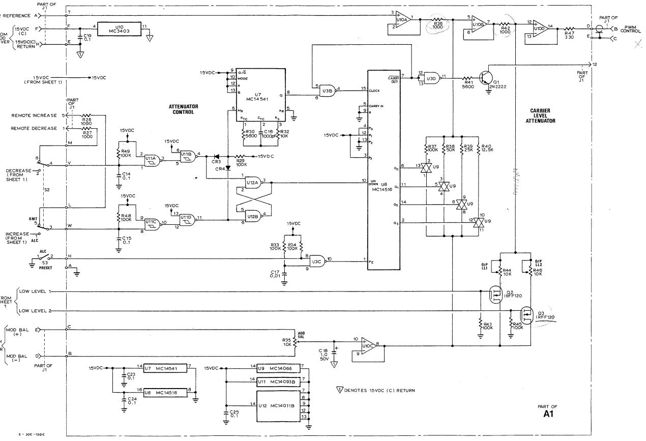
Figure FO-3 Electrical Schematic - NAPC18 ALC Power Trim Module (Sheet 2 of 2)
